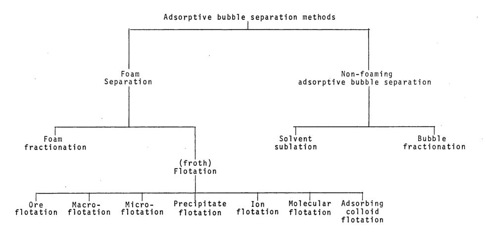
adsorption at the bubble surfaces. Froth flotation, or simply flotation (26), is the removal of particulate material by frothing (foaming).
