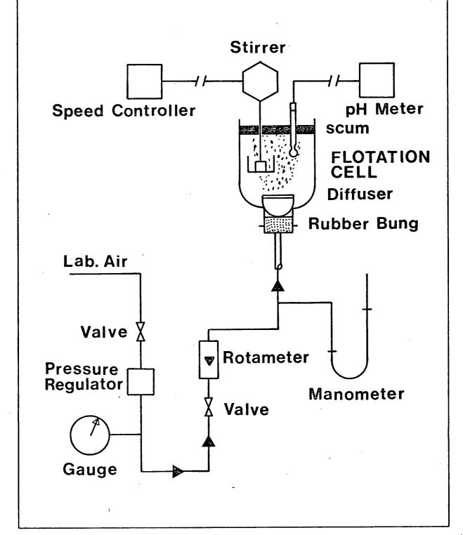
11.5 cms from the top of the vessel by means of a rubber bung, which also sealed the bottom of the cell. The froth was removed manually with a small scoop.
