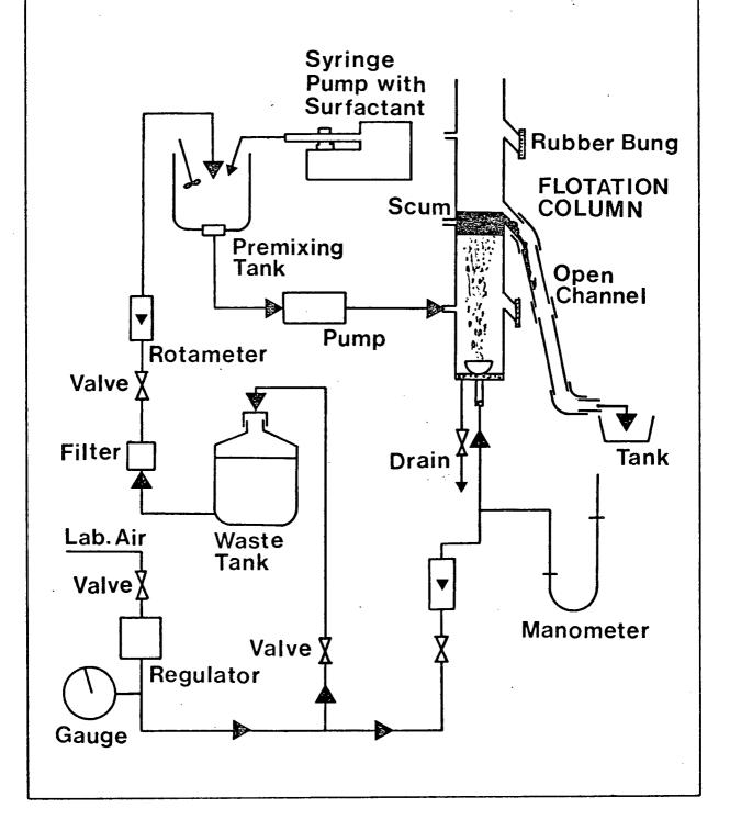
was prepared in a separate container and then added through a syringe pump. Both streams discharged into the top of the premixing tank.
