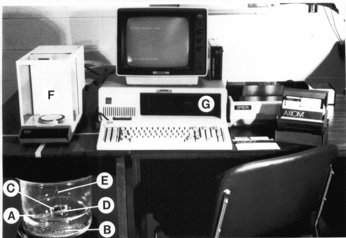
Figure VI-45. Experimental Setup for Water Absorption by Nylon Fibres.
