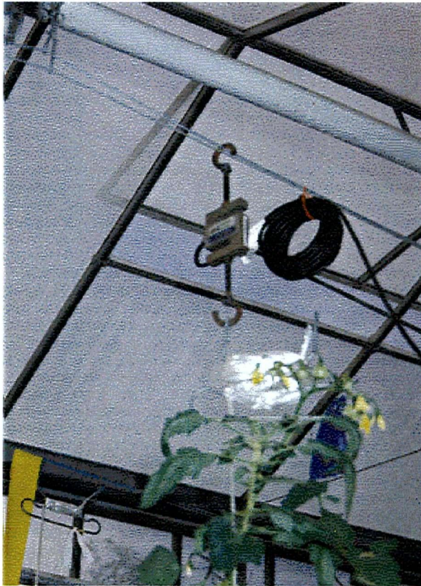
Figure 3-3 Sbeam load cell used to monitor plant weight
