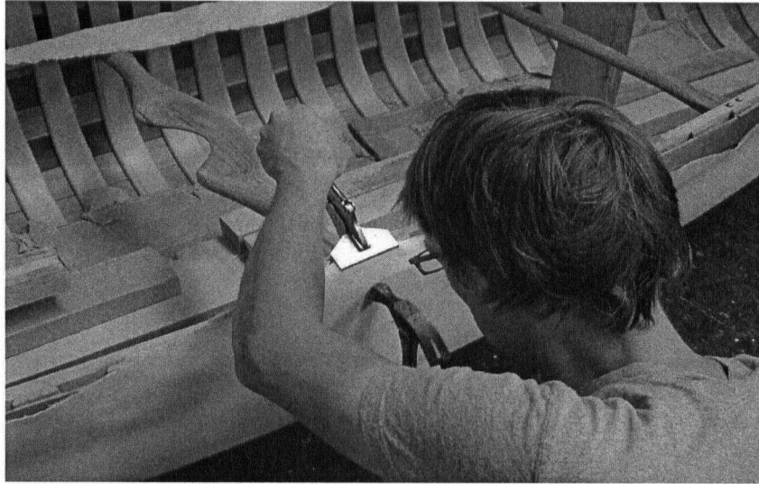
Figure 31. Tacking the canvas to the edge of the hull
