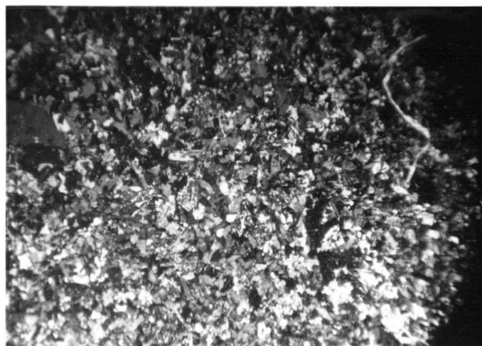
Figure 11. Texture of chilled granophyre. Fine-grained mosaic of quartz and potash feldspar. X47.
