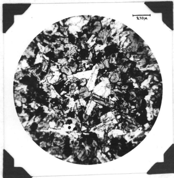
Plate 10: Fresh diabase, consisting of pigeonitic pyroxene (grey), labradorite (white) and magnetite (black) Compare with plate 9. Crossed nicols.
