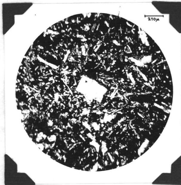
Plate 11: Fresh diabase, showing crudely-porphyrritic, contact facies, with phenocrysts of pyroxene and feldspar in a fine matrix of the same minerals and magnetite. Some feldspar is zoned. Crossed nicols.
