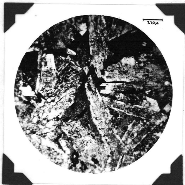
Plate 9: Late diorite dyke, consisting mainly of secondary green to brown amphibole (dark) and andesine feldspar (light). Compare with plates 10 and 11.
