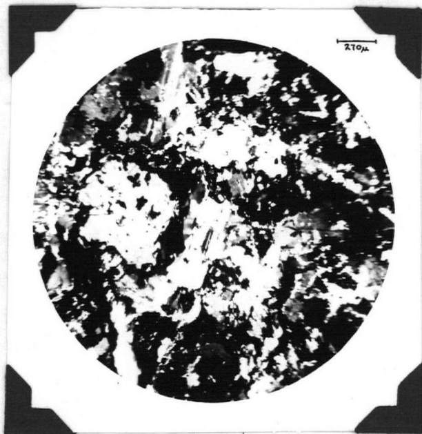
Plate 7: Unsheared "metadiorite". Note lack of any directive texture. Rock composed mainly of albite (white) and chlorite (black), with minor quartz, carbonate, sericite and apatite. Crossed nicols.
