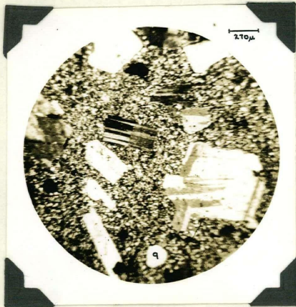
Plate 3: Porphyritic Rhyolite flow or quartz-feldspar porphyry intrusive. Phenocrysts are albite and quartz (q) in a fine-grained, holocrystalline matrix of quartz and feldspar. Crossed nicols.
