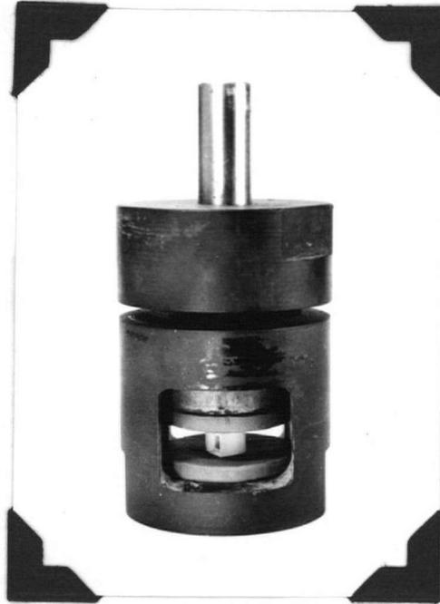
Figure 2. Vise Assembled for Bomb Run, with Static Loading Bar in Place
