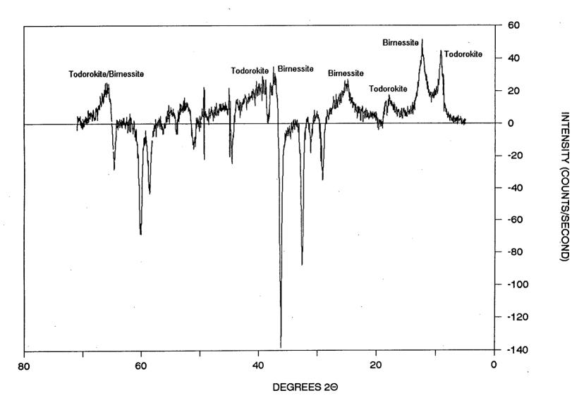
Figure 3-27. The DXRD pattern obtained after the first stage of leaching of the sequential extraction scheme on the Mn-enriched hydrothermal nodules.
