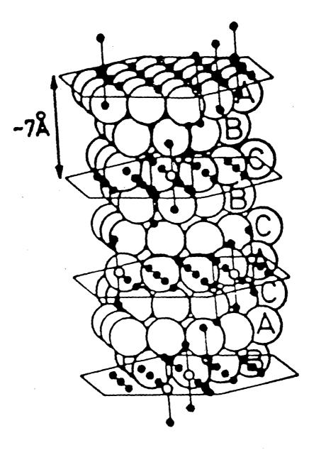
Figure 3-38. The crystal structure of  $\delta MnO_2$  (modified from Giovanoli *et al.*, 1965).
