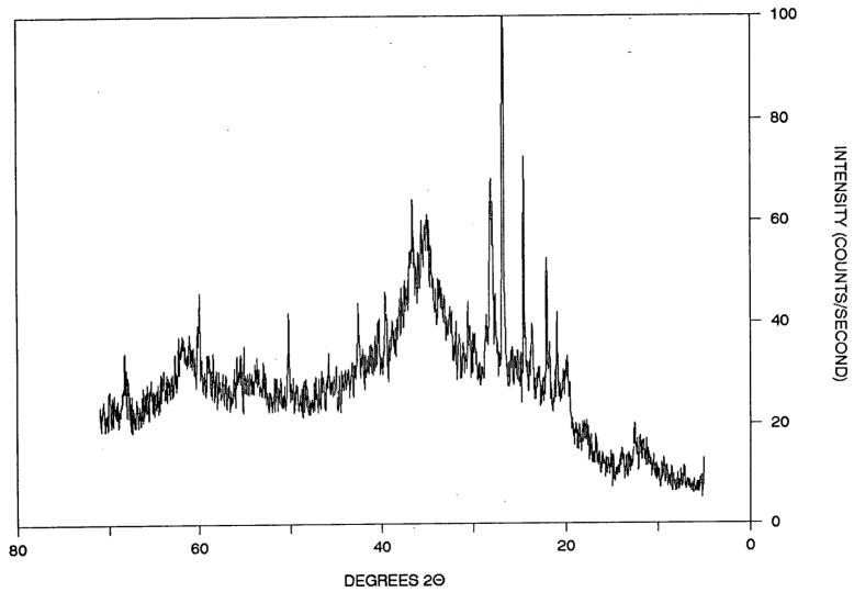
Figure 2-6. The DXRD pattern obtained after the first stage of leaching of the sequential extraction scheme on the laboratory standard crust DODO 14 DZ.
