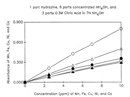
calibration lines. An aliquot of the leachate was diluted 500 times by measuring  $10\mu$ L of leachate and 4.99mL of the same reagent used in the experiment into an acid washed 5mL test tube. The test tube was capped and shaken vigorously to ensure sample homogeneity. The concentration of Mn, Fe, Cu, Ni, and Co in the leachate was then determined by plotting their measured absorbance values onto calibration curves. The reslts of these analysis are given in Appendix A.
