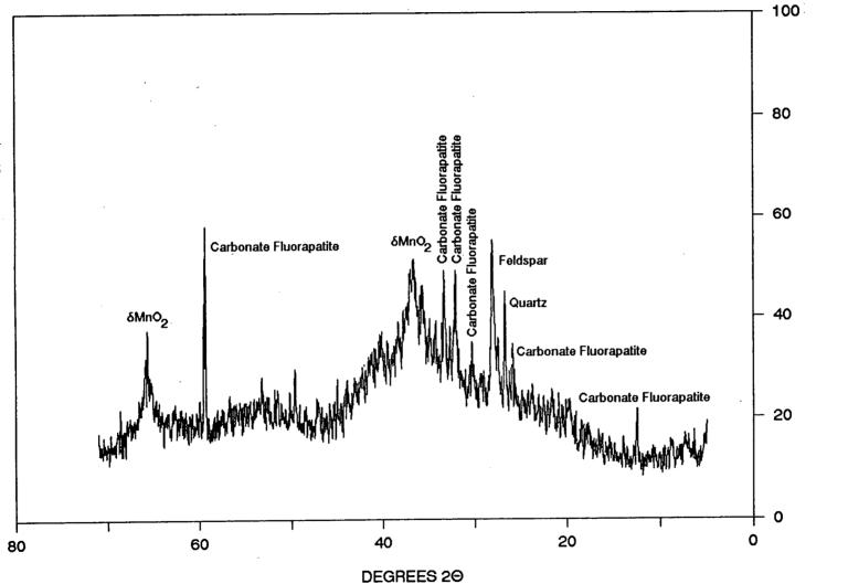
Figure 3-6. The XRD patterns of diagenetic nodules selected for the two stage selective sequential extraction scheme.
