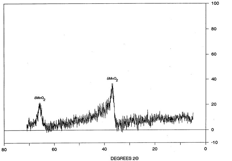
Figure 3-18. The DXRD pattern obtained after the first stage of leaching of the sequential extraction scheme on the hydrogenous nodules.
