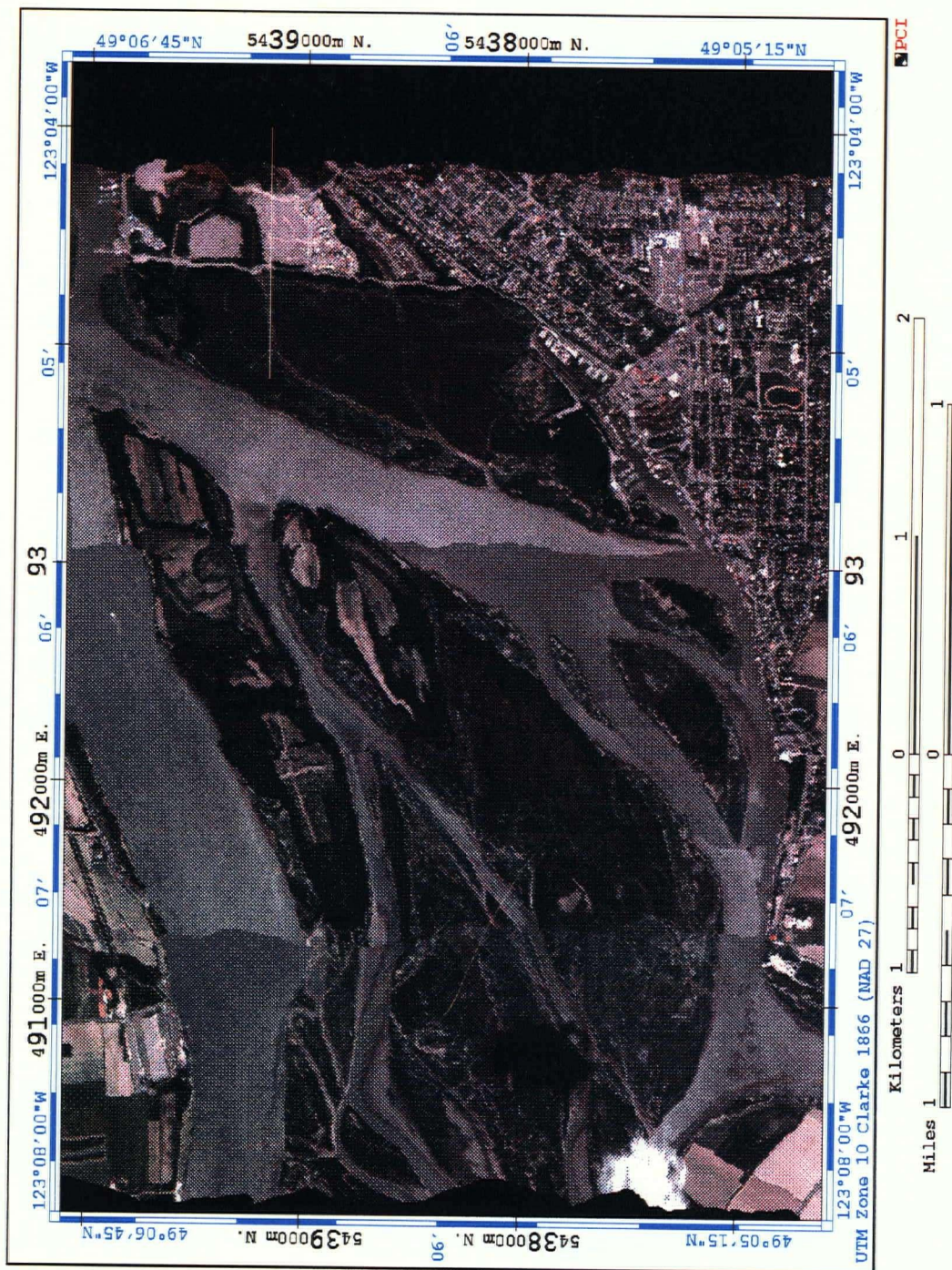
Fig. 4. Image mosaic of the South Arm Estuary, June 1992. Displayed bands are 6 (658-670 nm), 3 (545-556 nm), and 1 (450-503 nm).
