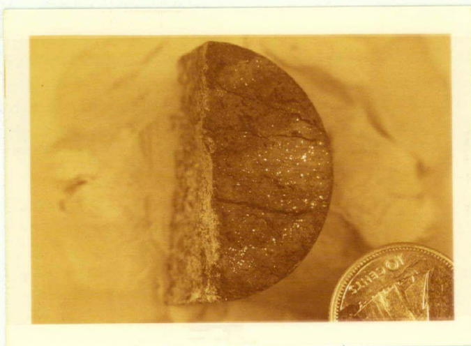
Figure 17: Chalcocite in drill core x 2 Dark bands are gypsum.
