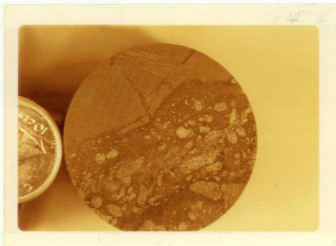
Figure 10. Agglomerate dyke at siltstone contact, X 1\frac{1}{2} .
