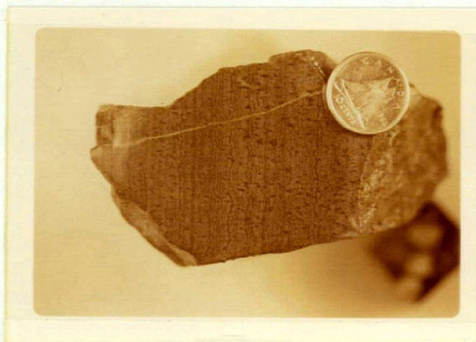
Figure 12: Polished specimen from No. 1 Cupriferous bed. Dark spots cutting laminae are sulfides.
