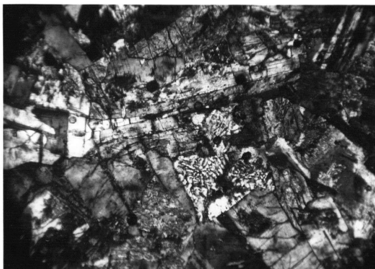
B--Photomicrograph of quartz diabase showing micrographic intergrowths of quartz and plagioclase. Polarized light X47.
