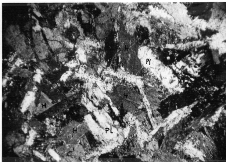
B--Photomicrograph of amphibolite showing relict ophitic texture. Lot 3, concession B, Steele township. H= hornblende, Pl= plagioclase. Also present are chlorite, epidote, quartz and opaque minerals, Polarized light X16.
