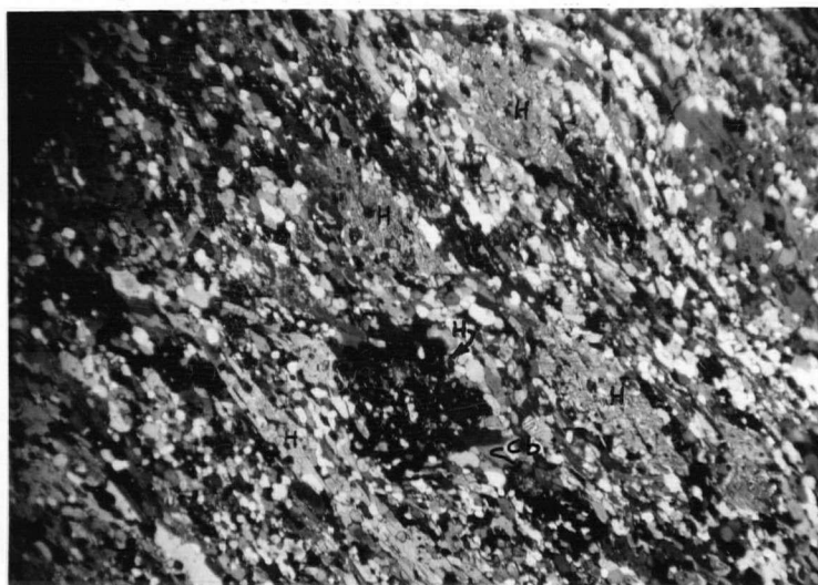
B--Photomicrograph of schistose amphibolite, lot 12, concession V, Bonis township. Sieve-textured hornblende (H), containing inclusions of quartz and carbonate (Cb) lie in a groundmass of quartz, plagioclase and epidote. Polarized light X16.
