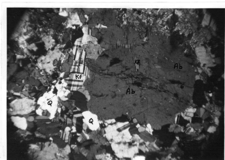
A--Photomicrograph of quartz monzonite showing K-feldspar (Kf) replaced by albite (Ab). Lot 3, concession IV, Bonis township. Quartz (Q) hornblende, biotite, epidote, sphene and apatite are also present. Polarized light X47.
