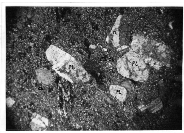
Photomicrograph of feldspar porphyry, lot 6, concession E, Steele township. Twinned, altered plagioclase phenocrysts (Pl) lie in a fine-grained matrix of quartz, feldspar, sericite, chlorite, and carbonate (Cb). Polarized light X16.
