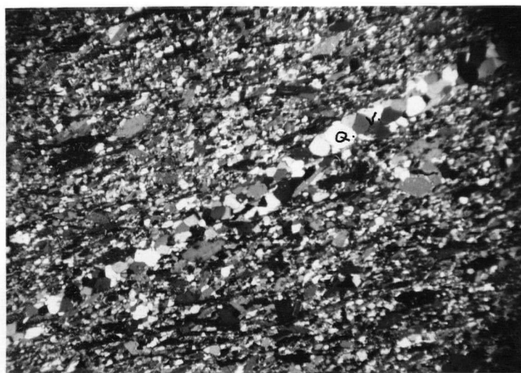
B Photomicrograph of a quartz veinlet (Q.V.) in sheared greywacke. Lot 5, concession II, Steele township. The rock consists of quartz, albite, muscovite, and biotite. Polarized light X16.
