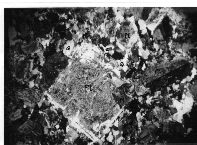
B--Photomicrograph of granodiorite showing an altered zoned plagioclase crystal. Lot 1, concession D, Steele township. Pl= plagioclase, Q= quartz, M= muscovite, Kf= K-feldspar. Epidote, chlorite, apatite and sphene are also present. Polarized light X16.
