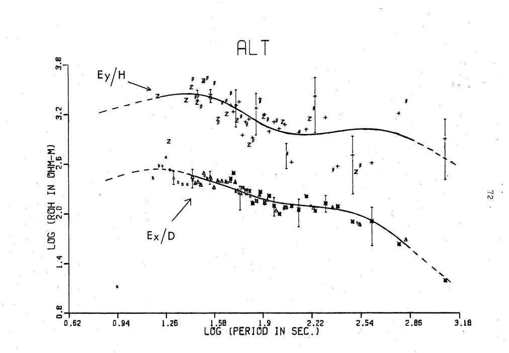
Apparent resistivity curves at Pemberton. The symbols + and \* correspond to W1, (3 and  $\Delta$  correspond to W2, Z and O correspond to W3, where W stands for the smoothing window. The vertical bars represent one standard deviation.
