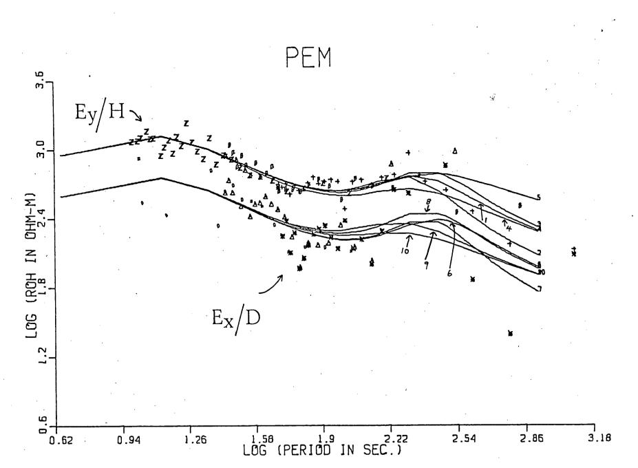
Computed apparent resistivity model curves (solid lines) drawn on the experimental data (symbols) at D'Arcy.
