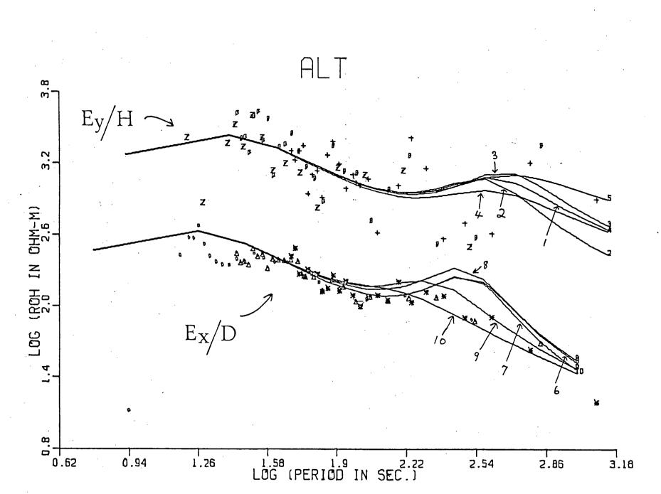
Computed apparent resistivity model curves (solid lines) drawn on the experimental data (symbols) at Pemberton.
