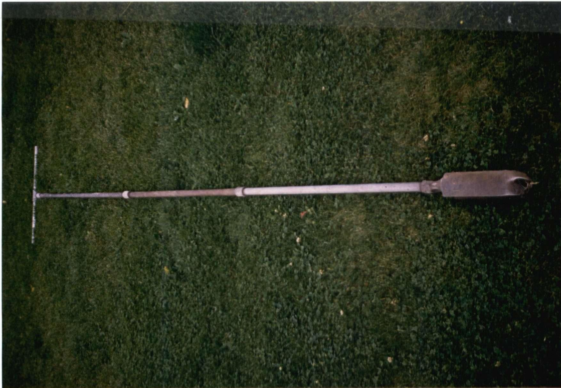
Plate A-2 Rotating dutch auger used to dig boreholes, 3m long with extensions
