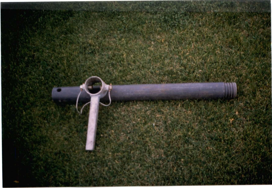
Plate A-5 3-inch internal diameter PVC casing used during deep piezometer installation. The apparatus used to remove the casing lies on top of it.
