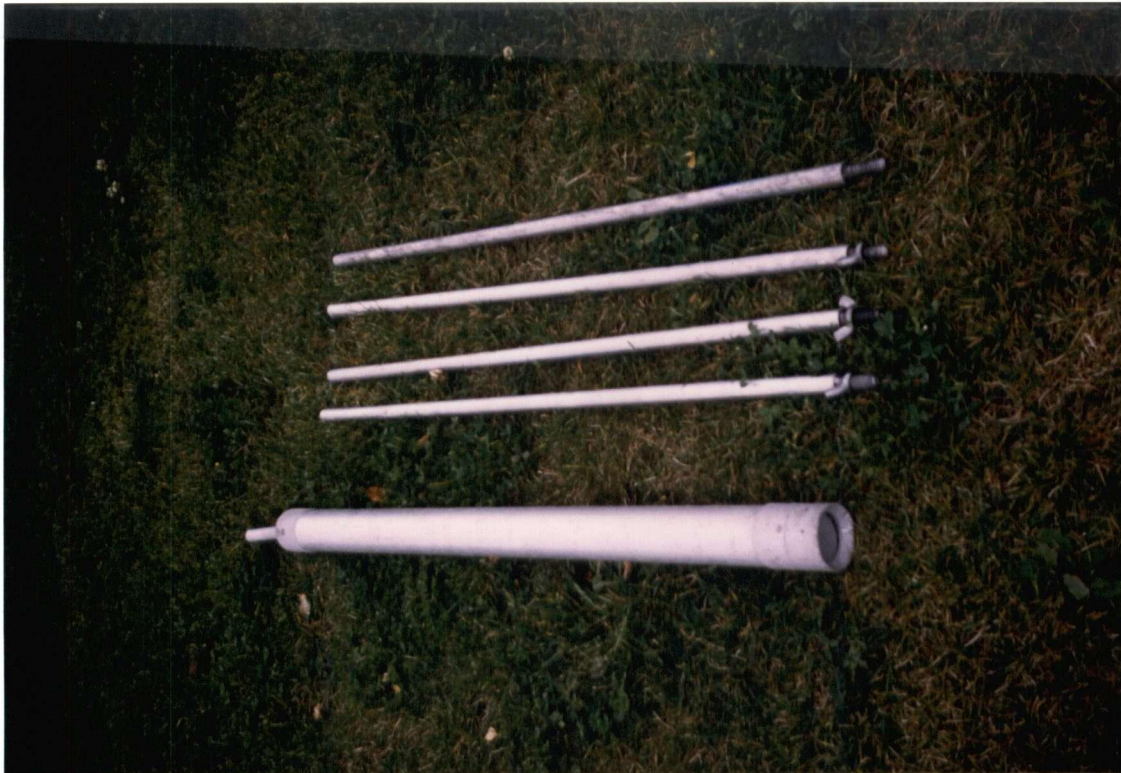
Plate A-4 Sand bailer with 1m-long extensions
