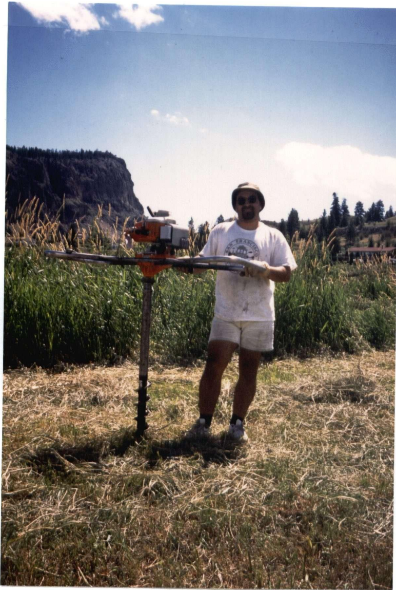
Plate A-3 Gas-powered post-hole digger
