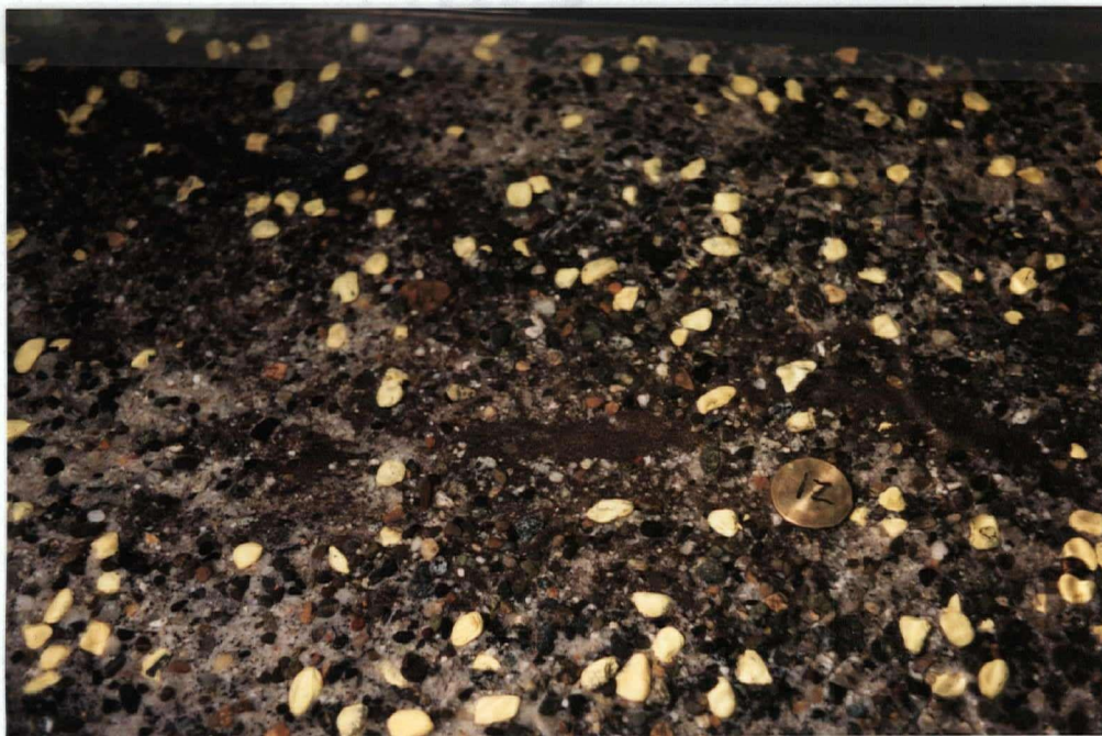
Figure 4-12. Run 5 concentrations of cassiterite after 10 min of flooding. Photo taken at 3.7 m with flow from left to right. Scale is given by the brass disk, 3.0 cm in diameter.
