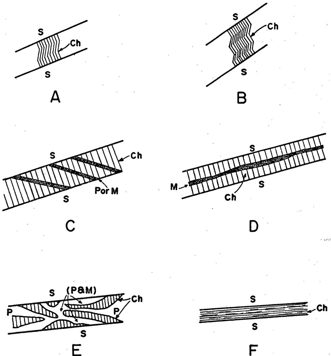
FIGURE 4-1: CHRYSOTILE-FIBRE VEINS.
