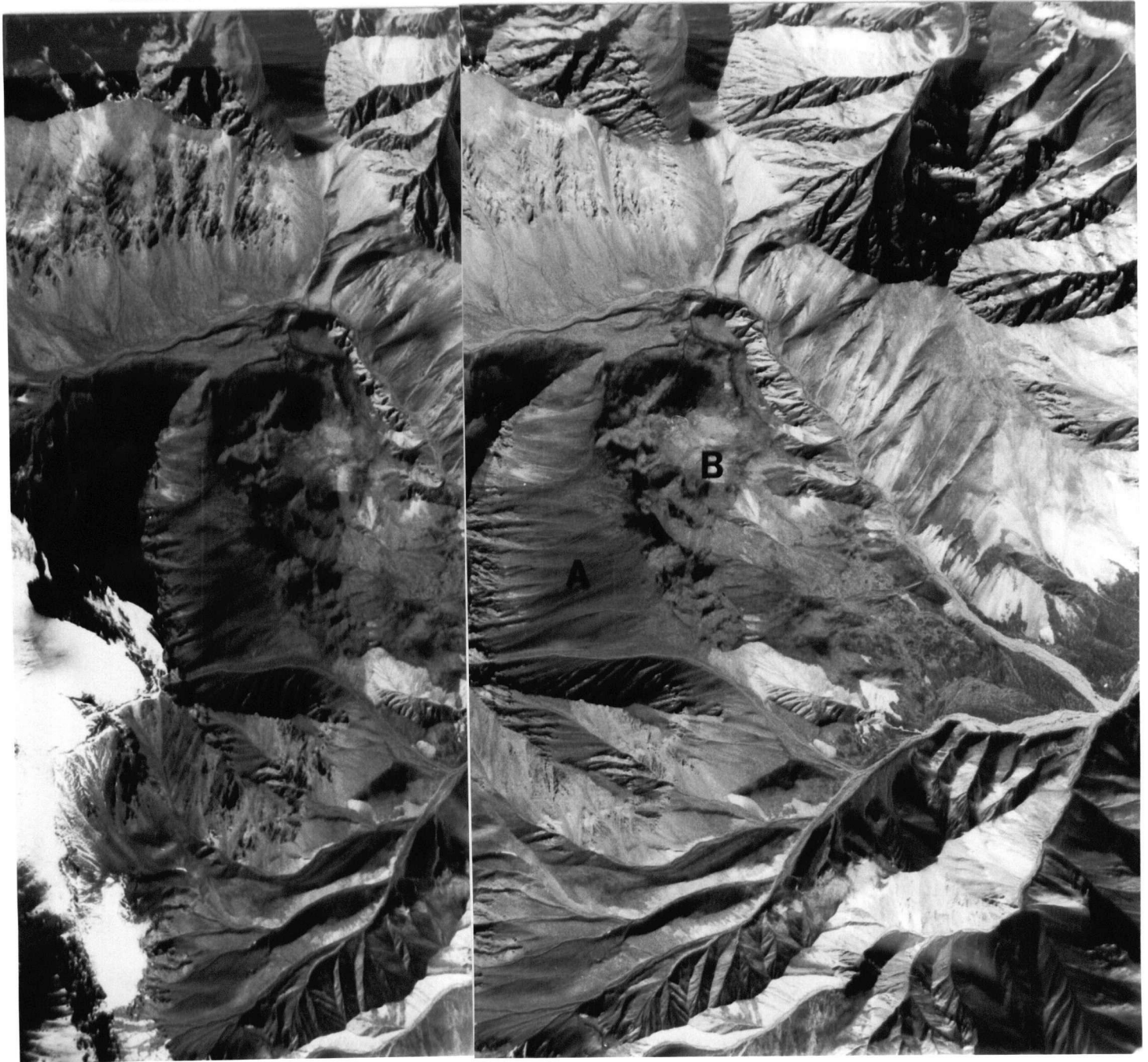
Plate 3.3. Nines Creek Rock-Block Slide. The slide block (B) has translated as a coherent wedge. Debris avalanches off the flank of the block post-dating the original movement are seen below (B) and to the right. The rupture surface (A) is a remarkably planar feature.
