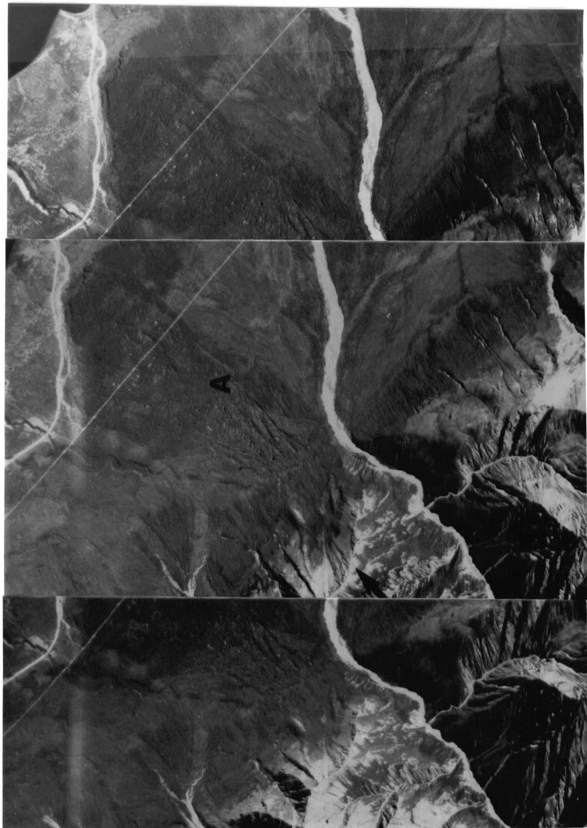
Plate 3.2. Congdon Creek Rock Avalanche. Hummocky debris (A) is conspicuous on the surface of Congdon Creek alluvial fan; note the contorted ridges at the base of the slope. The suspected source area is indicated by the arrow.
