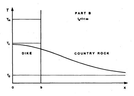
Figure 49: Coordinate system after solidification
