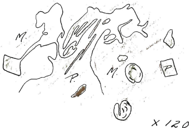
Fig. A. Camera lucida drawing of section from June Mine, showing forms of pyrite (P) replacing pyrrhotite (M). The tendency to develop idiomorphic form is noticeable. The spherical structure seen in the two grains was noted in several places, but it could not be explained.
