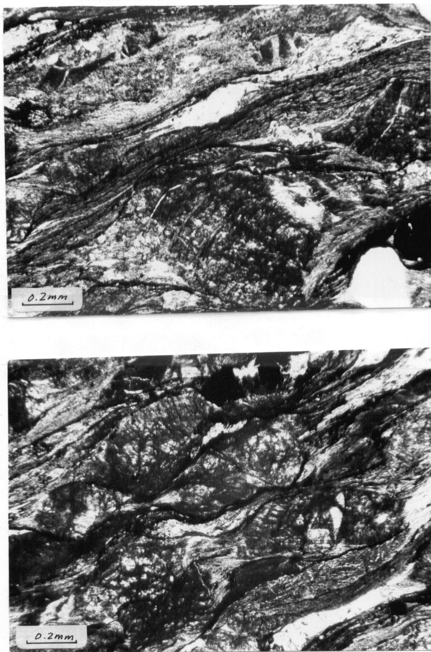
Figure 17. Photomicrographs of protomylonitized Cache Creek Group greywacke. Note shattered feldspar grains and fluxion texture in much of the matrix. Plane polarized light.
