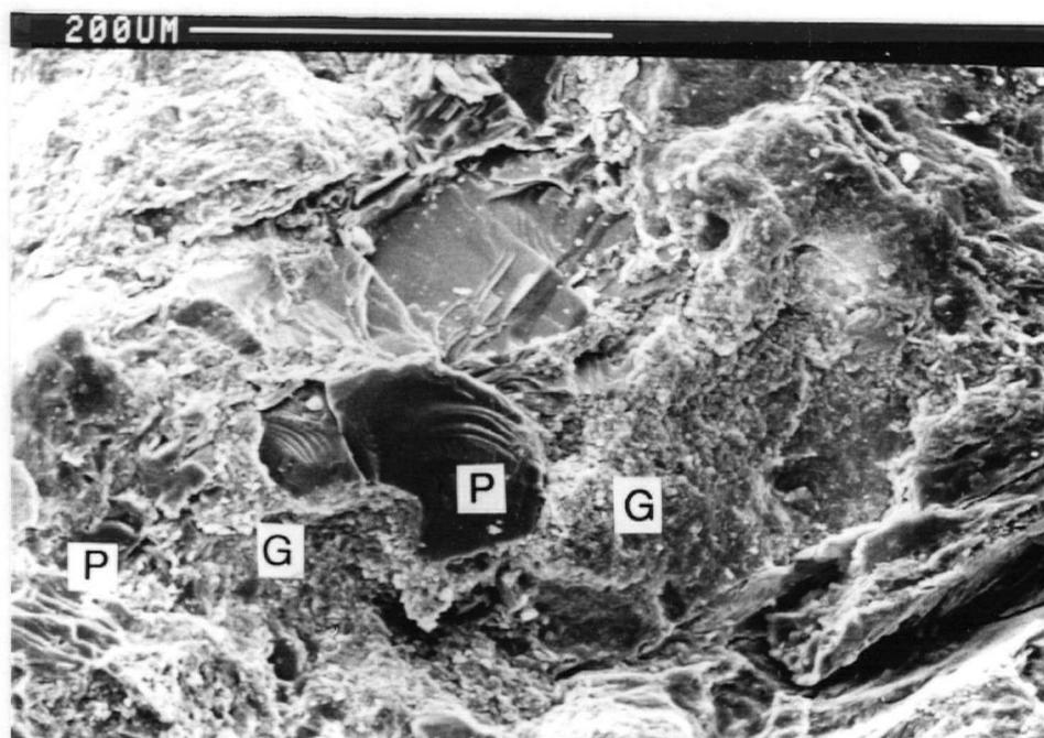
**Figure 2-8.** This SEM-photomicrographs shows that porosity is almost nonexistent in these glauconite rich sandstones (glauconite (G), plagioclase (P)).
