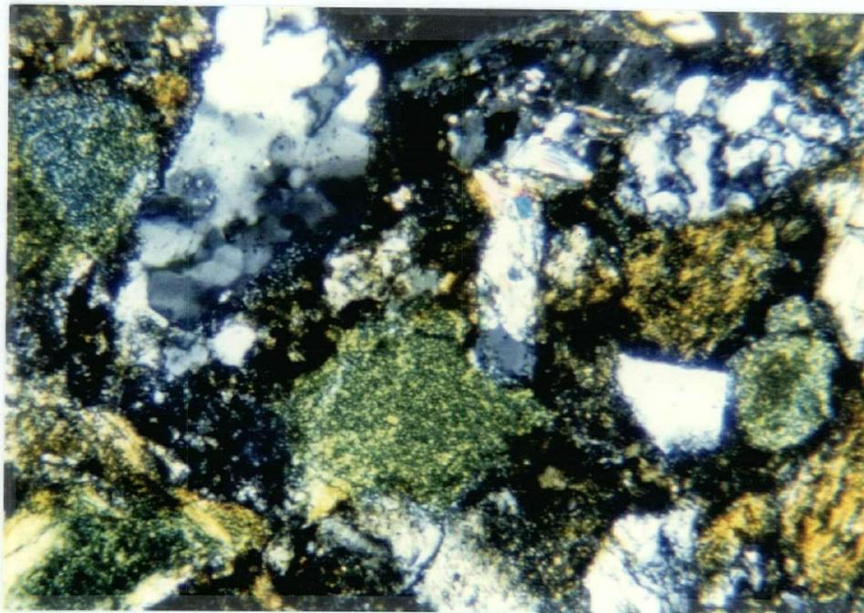
**Figure 2-6.** a) Thin section photomicrograph of sandstone rich in green glauconite fragments (plane polarized light , x70 magnification). b) Thin section photomicrograph of glauconite grain (crossed nicols, x280 magnification).
