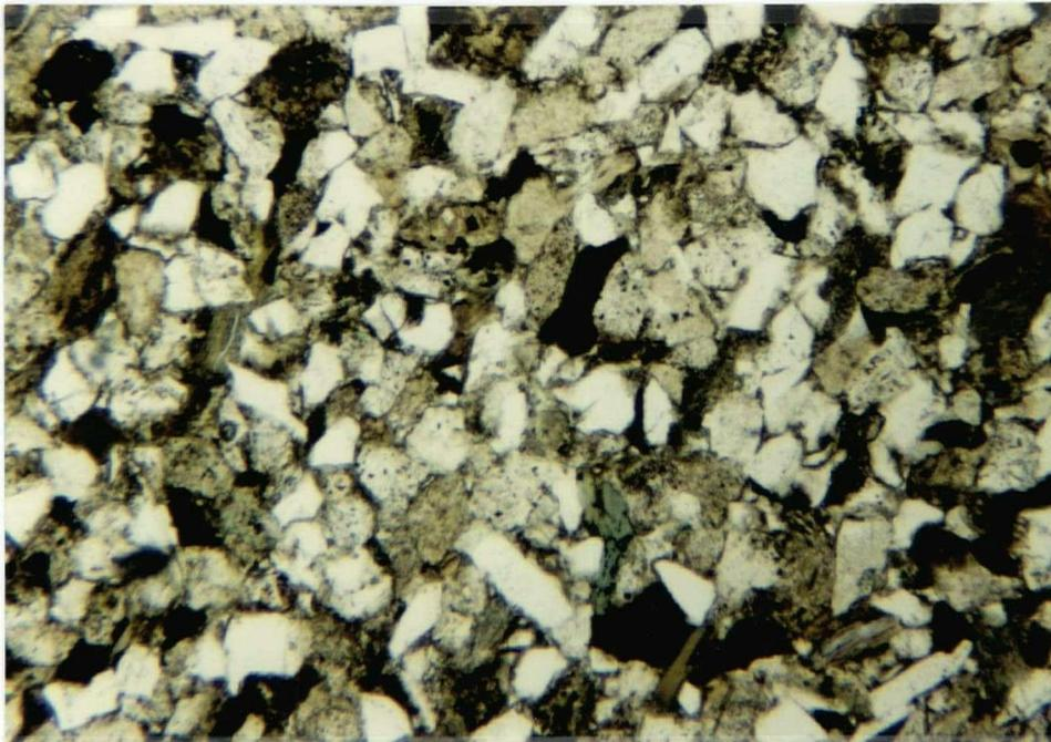
**Figure 2-4.** Thin section photomicrograph showing angular quartz and feldspar fragments in the massive sandstone lithofacies (plane polarized light, x70 magnification).
