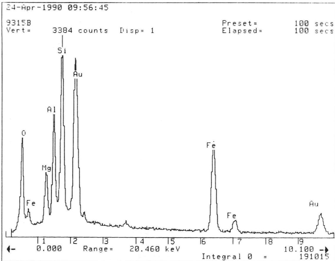
**Figure 2-9.** a) SEM-photomicrograph of chlorite (Ch), Carbonate (Ca), and rock fragment (RF). b) EDS-analysis of the chlorite grain in (a).
