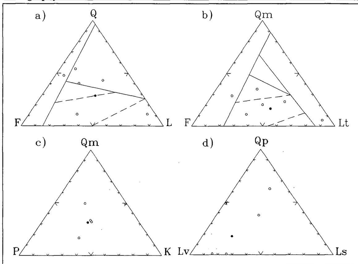
**Figure 2-5.** Ternary diagrams showing the relative abundance of a variety of different fragments in thin sections of the massive sandstone lithofacies (see appendix 7.1 for explanation to the abbreviations used in this diagram). a) QFL-diagram, b) QmFLt-diagram, c) QmPK-diagram, and d) QpLvLs-diagram (from Dickinson, 1982; Dickinson et al., 1982). Solid circles represent the average.
