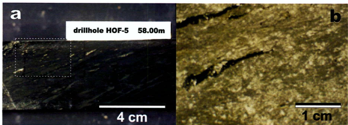
Plate 4.6. Basaltic flow tops from drill hole HOF-5, 58 m (Appendix 9).
