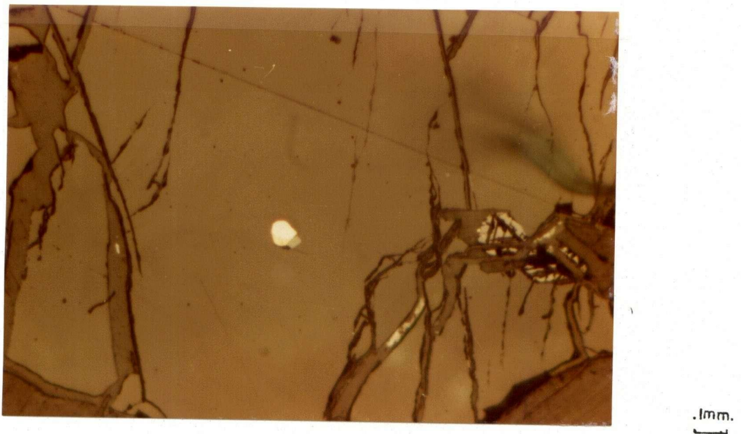
Fig. 15. Composite po.-cpy. bleb and magnetite grain enclosed in olivine. X63, plain light.
