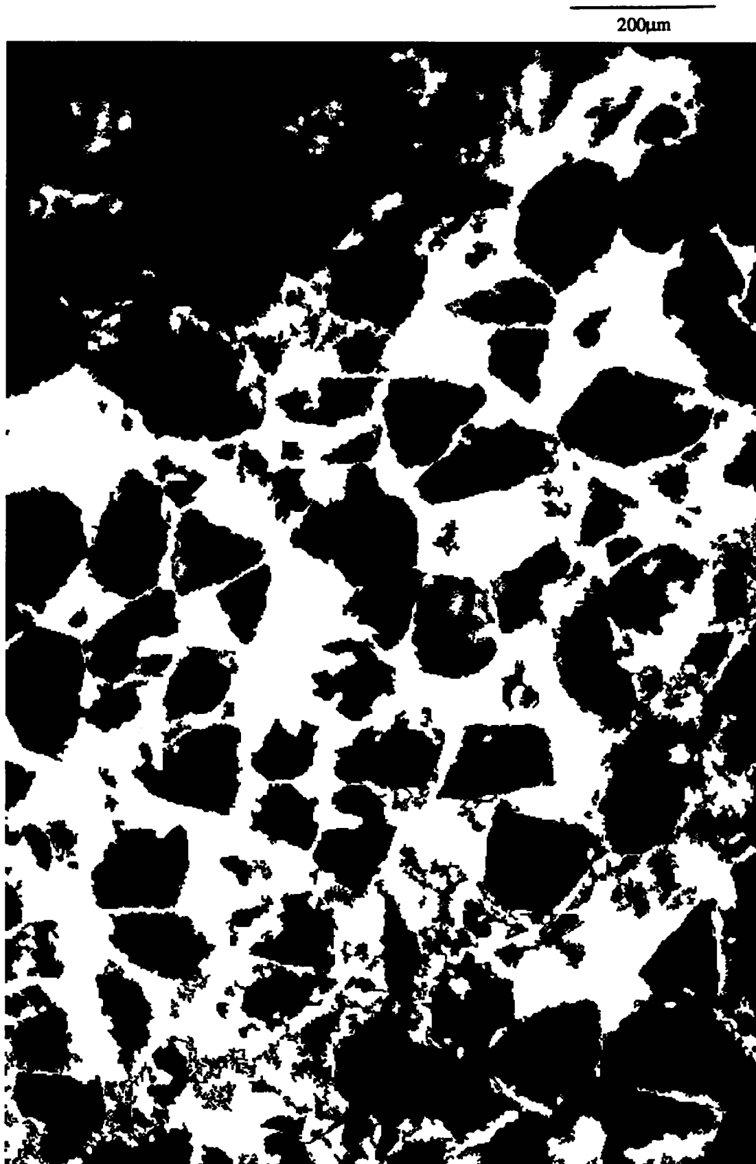
Figure 2.2a: Binary versions of Berea 100 image ABR1 with pore/solid separation value of 40. Black = solid, and white = pore space.
