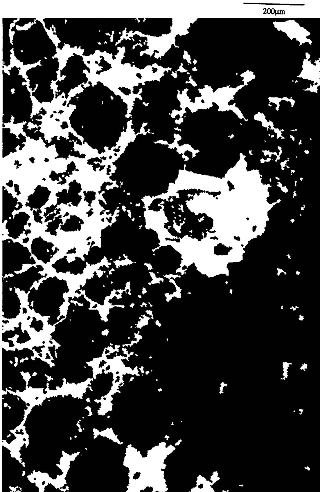
Figure 2.6b: Binary version of carbonate S55 CLSM image F78 (Figure 2.4a) produced using a solid/pore separation value of 100. White = porosity, and Black = solid.
