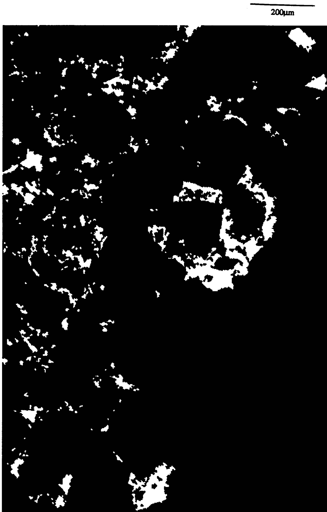
Figure 2.6a: Binary version of carbonate S55 CLSM image F78 (Figure 2.4a) produced using a solid/pore separation value of 50. White = porosity, and Black = solid.
