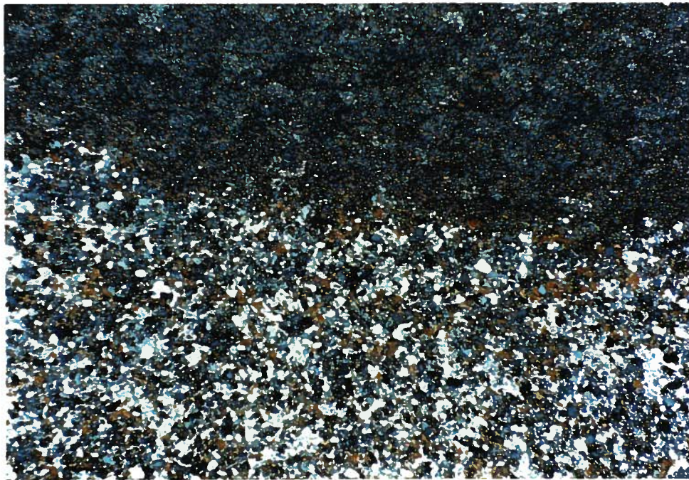
Plate 4.2: Photomicrograph (transmitted light, crossed polars, field of view = 5.0 mm) of biotite + cordierite altered argillite and siltstone from the Apex Mountain complex (unit 1: Fig. 4.1).
