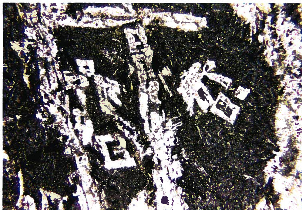
Plate 4.22: Photomicrograph (transmitted light, crossed polars, field of view = 5.0 mm) of aphyric Hedley sill (unit 7: Fig. 4.4). Plagioclase crystals have altered glass cores. Such textures are described as "belt-buckle" texture (Bryan, 1972). Sample is from lower stope, French mine.
