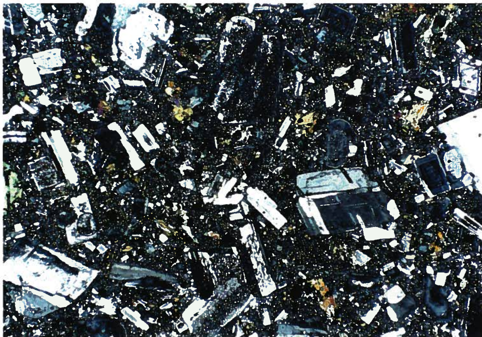
Plate 3.13: Photomicrograph (transmitted light, crossed polars, field of view = 5.0 mm) of andesite crystal tuff from the upper unit of the Skwel Peken formation (unit 13b: Fig. 1.1).
