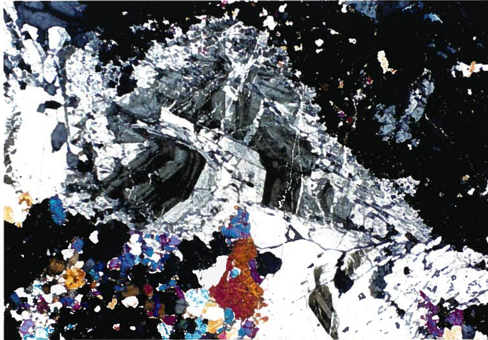
Plate 4.29: Photomicrograph (transmitted light, crossed polars, field of view = 5.0 mm) of optically zoned vesuvianite crystals in a vein cross-cutting garnet \pm clinopyroxene skarn. Protolith of this sample is likely Hedley formation limestone (unit 2: Fig. 4.4). Sample is from the lower stope, French mine.
