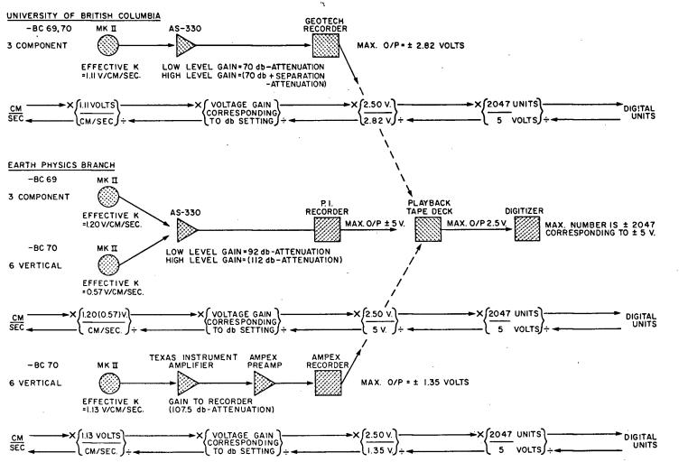
Fig. 4 The system factors for conversion of ground velocity to digital units and back to ground velocity. Note effective K applies to passband centre only.
