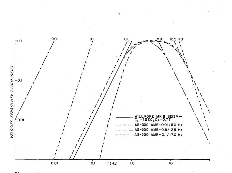
Fig. 3 The response curves of the systems shown in Fig. 2.
