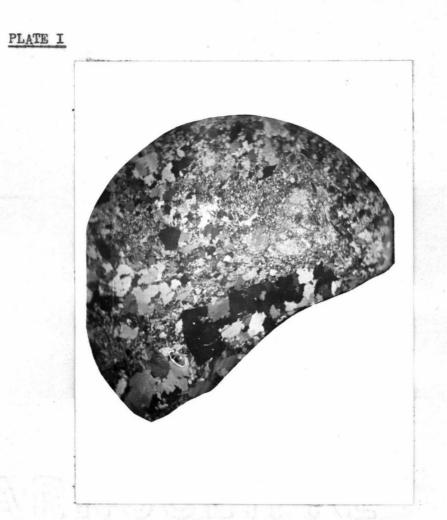
Rock Fragment: the form and size of this fragment can be clearly seen in this picture. Several smaller fragments can be seen but not so clearly. An idea of the fairly fine grained groundmass and the abundance of quartz typical of all specimens can be obtained from this picture. Slide 9, Specimen 20 X nicols
