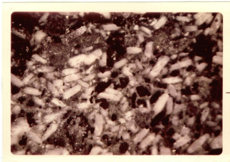
PLATE VII LOBE DIORITE PORPHYRY (X-6) Subtrachytoid texture.
