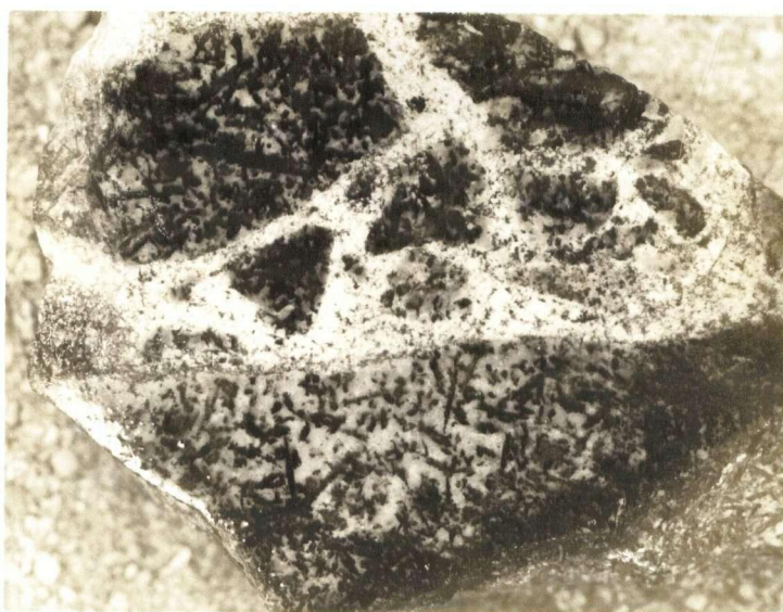
PLATE II AJAX BRECCIA (X- \frac{1}{2} ) Fragments of Iron Mask Diorite in Microdiorite matrix.
