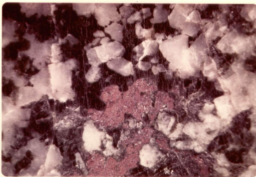
PLATE I IRON MASK GABBRO (x-6) Note the ophitic texture, and hematite (red) after magnetite.
