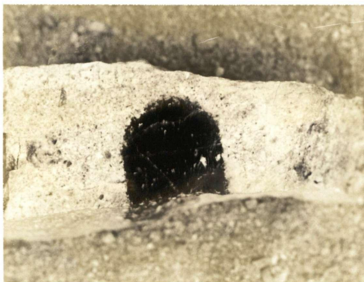
PLATE XIV AJAX BRECCIA (X-1) Fragment of Iron Mask Gabbro in strongly propylitized Microdiorite.
