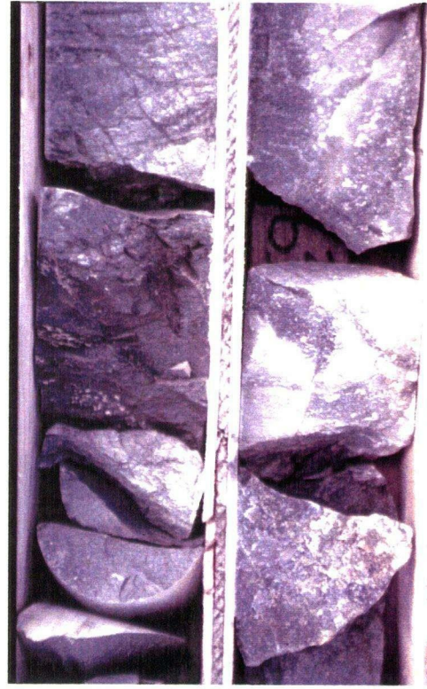
Plate 4.20. Silicified quartzite (unit 1a) hosting quartz-sulphide stringer stockwork.
