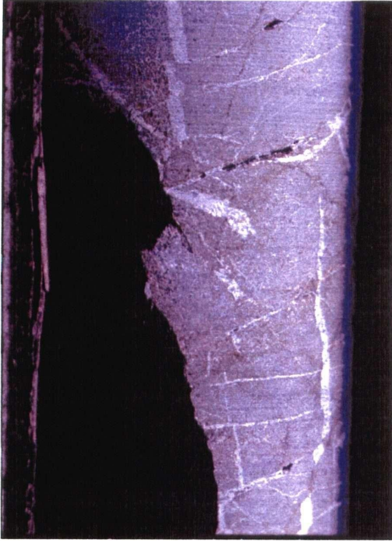
Plate 4.14. Moderate dolomitization of ooids in MSLT. HQ core. Core diameter = 61 mm.
