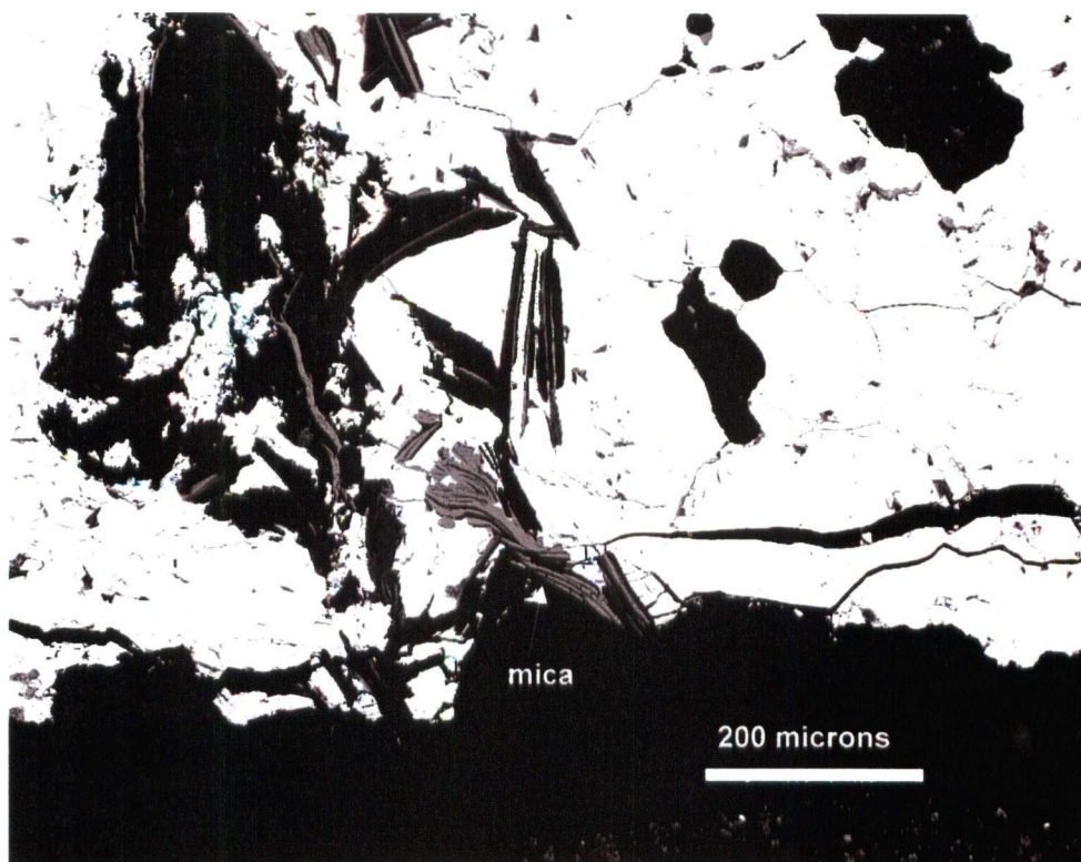
Plate 6.2. SEM image of fine-grained muscovite (intermediate gray) intergrown with quartz (black) and sulphides (white) in carbonate hosted manto style mineralization. Sample 4448.
