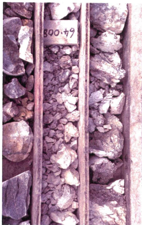
Plate 4.6. Brecciated quartz vein in core. HQ core. Core diameter = 61 mm.
