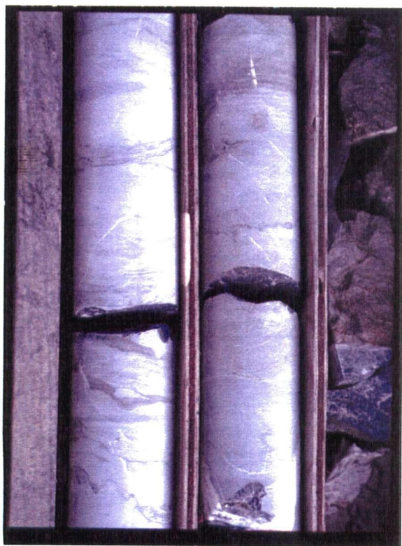
Plate 2.5. WBN facies (unit 1d) - light gray, sparsely silty banded lime mudstone. NQ core. Core diameter = 45 mm.
