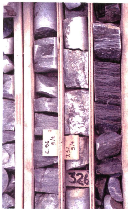
Plate 4.12. Mineralized quartz-sulphide vein in calcareous quartzite. HQ core. Core diameter = 61 mm.
