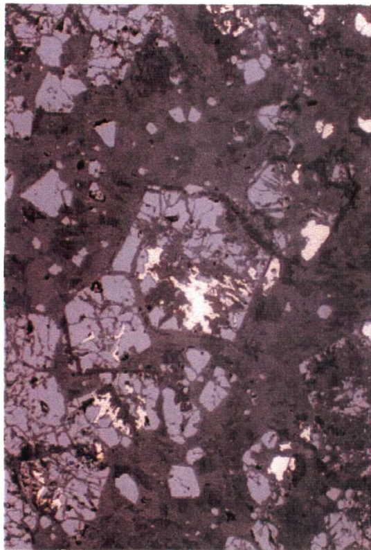
Plate 4.28. Euhedral magnetite (gray) replaced by pyrite (yellow), and cross-cut by quartz and muscovite (dark gray). Field of view = 1 mm.
