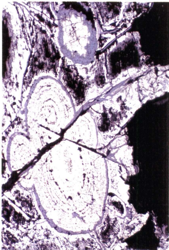
Plate 4.32. Late, colloform marcasite. Field of view = 2 mm.
