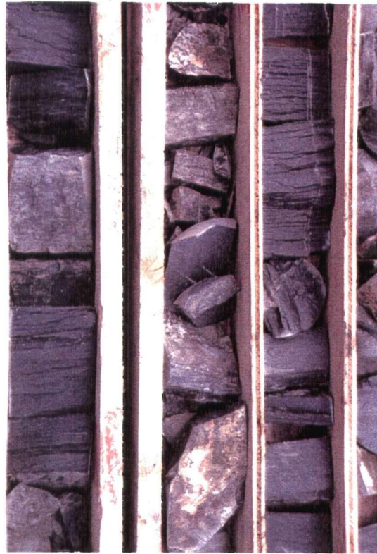
Plate 2.3. M-PHYL - black phyllite is the most conspicuous marker within unit 1a. HQ core. Core diameter = 61 mm.
