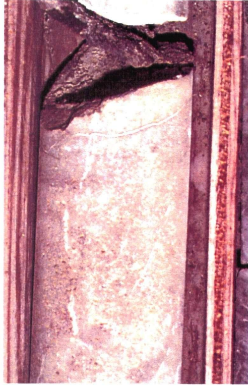
Plate 4.16. Strong decalcification (porous core) and dolomitization. HQ core. Core diameter = 61 mm.
