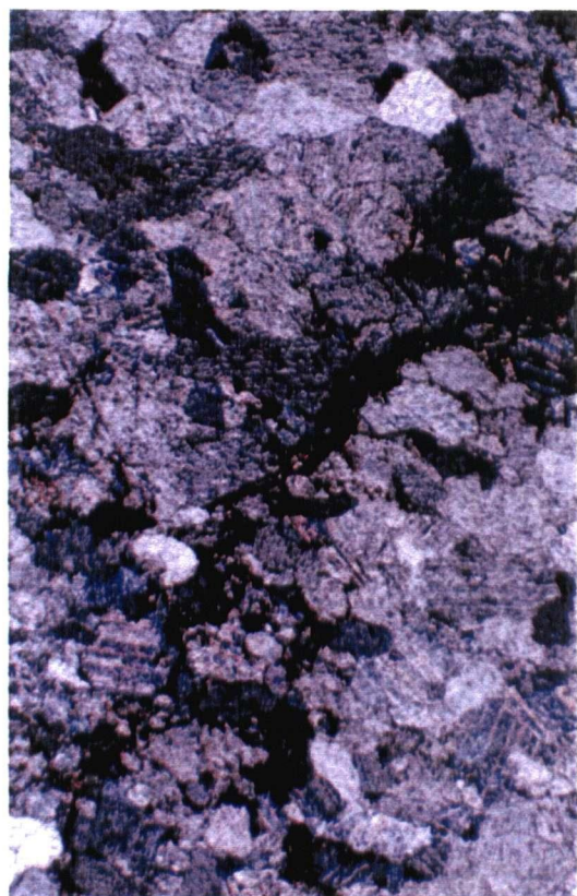
Plate 2.6. Secondary fracture enhanced porosity (12%) in WBN. Field of view = 1 mm.
