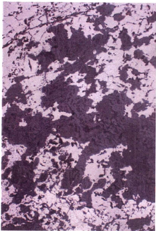
Plate 4.36. Fine-grained muscovite (light gray) intergrown with quartz (dark gray) and pyrrhotite (yellow). Field of view = 10 mm.
