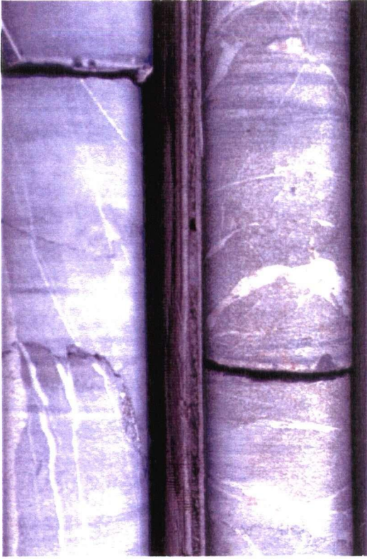
Plate 2.10. MSLT (unit 1d) - massive oolitic grainstone to packstone, with locally dolomitized ooids. NQ core. Core diameter = 47 mm.
