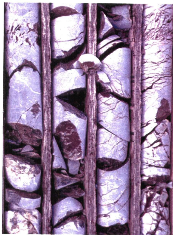
Plate 2.7. BXLT (unit 1d) - blue, coarsely crystalline dismicrite, with abundant fractures. NQ core. Core diameter = 61 mm.
