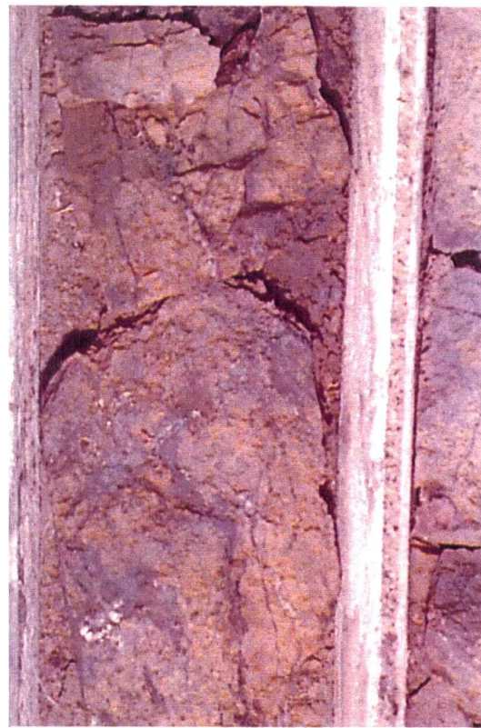
Plate 4.4. Oxide ore in core. HQ core. Core diameter = 61 mm.
