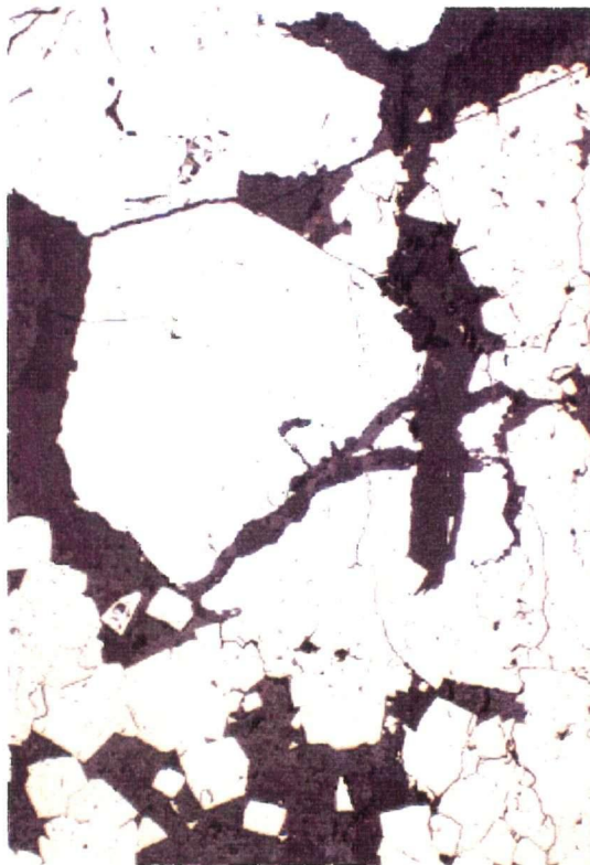
Plate 4.29. Early, euhedral arsenopyrite (white) cross-cut by quartz and muscovite (dark gray). Field of view = 2 mm.
