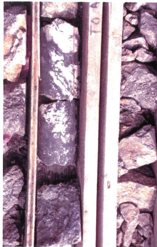
Plate 4.7. Quartz-arsenopyrite vein hosted in metasedimentary rocks (unit 1a). HQ core. Core diameter = 61 mm.
