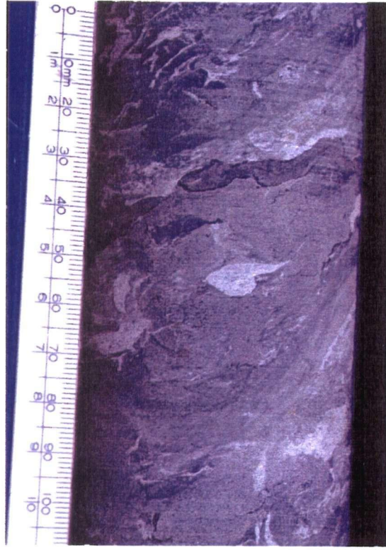
Plate 2.12. BSLT (unit 1d) - black, silty lime mudstone with soft sediment deformation features. HQ core. Core diameter = 61 mm.
