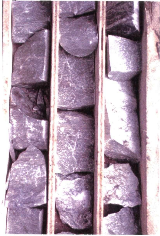
Plate 2.2. M-QZE (unit 1a) massive, light gray to white quartzite. HQ core. Core diameter = 61 mm.
