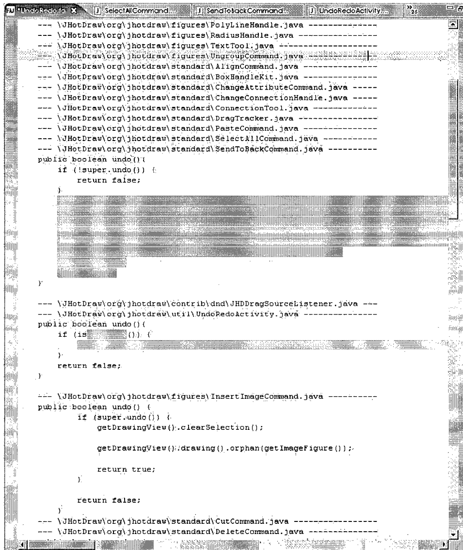
Figure 6.1: Part of the overlaid undo methods - the undo method in InsertImageCommand is inconsistent with the similar undo methods.
