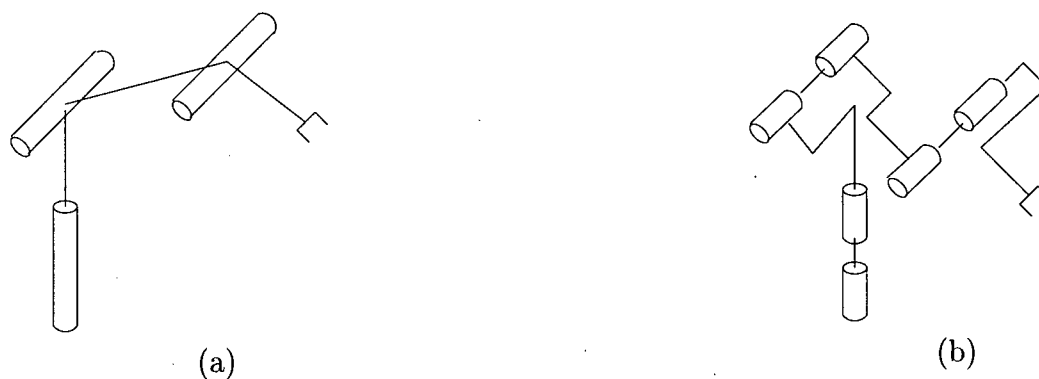
Figure 2.3: Depicted in (a) is a 3-R manipulator, and (b) a 6 DOF manipulator which is first-order fault tolerant. Each joint has a parallel joint which, in the event of a fault, can be used to position the arm. The example is modified from [PAK94] and is illustrative of designs found in [WDHC91].
