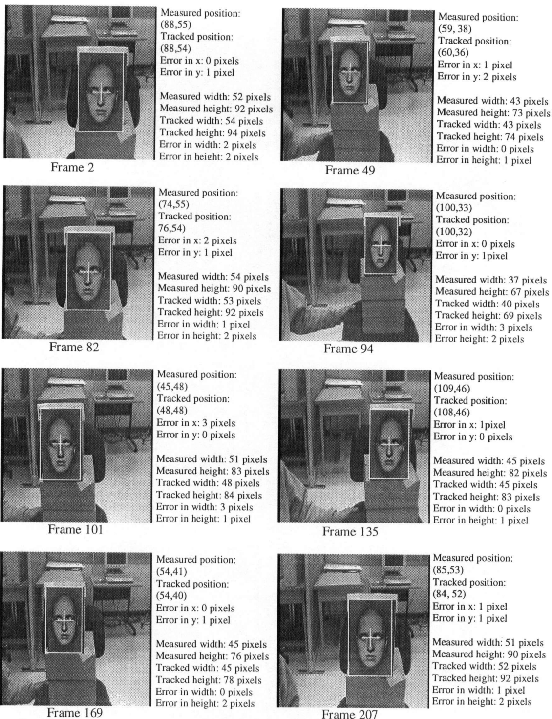
Figure 5-7 Tracking Accuracy - Translation Comparison between tracked and measured positions and sizes in multiple frames of a video sequence representing the tracking of the portrait of a head as it translates in the scene.
