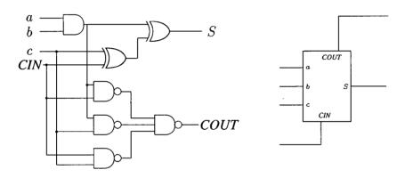
Figure 7.4: Base Module for Multiplier
