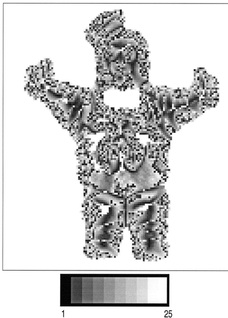
Figure 5.49: Translating Stay-Puft Marshmallow Man. Condition number for multiple light source optical flow.
