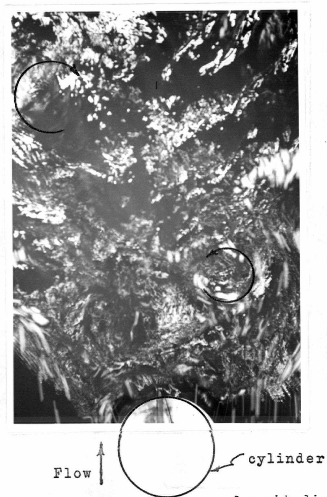
Fig. 38 Cylinder vibrating near longitudinal resonance
