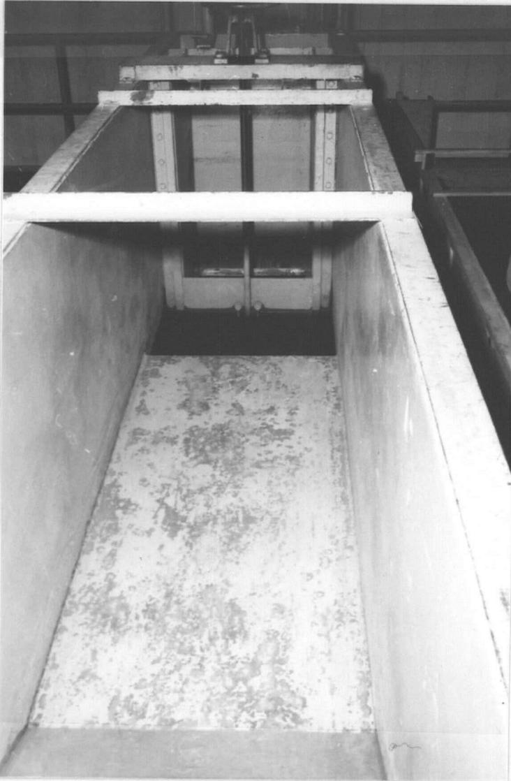
Fig. 36. Interior Detail of the 39'-4 $\frac{1}{4}$ " Long, 30" Wide and 36" Deep Flume in the Region Chosen for Installation of the Proposed New Wave Generator.
