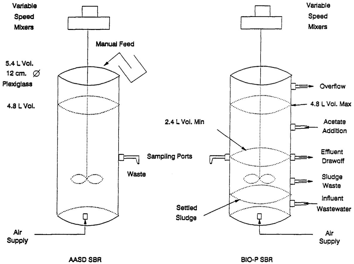
Figure 3.4 Schematic of AASD and Bio-P Sequencing Batch Reactors
