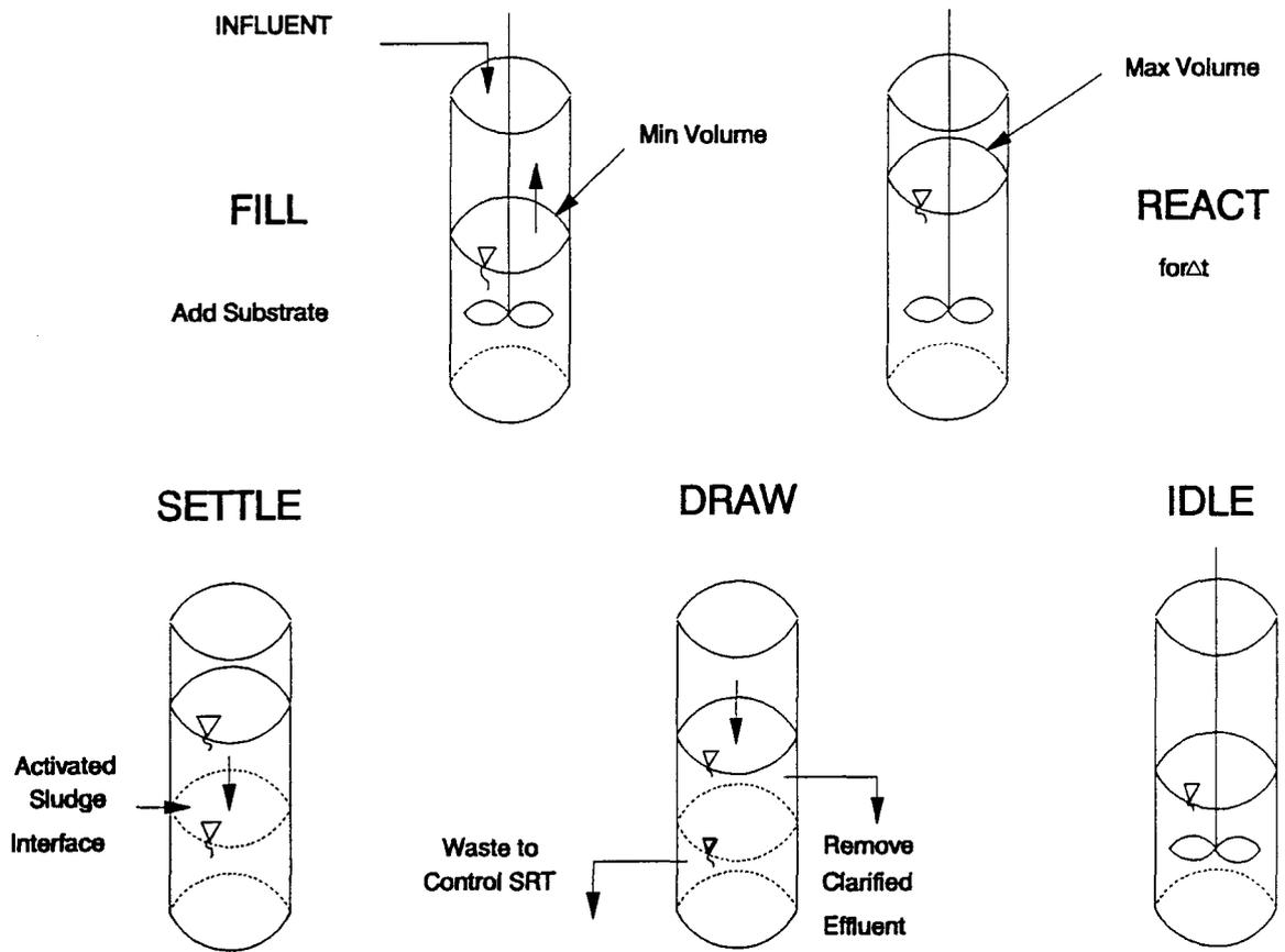
Figure 2.3 Diagram of 5 Operating Periods of Bio-P SBRs
