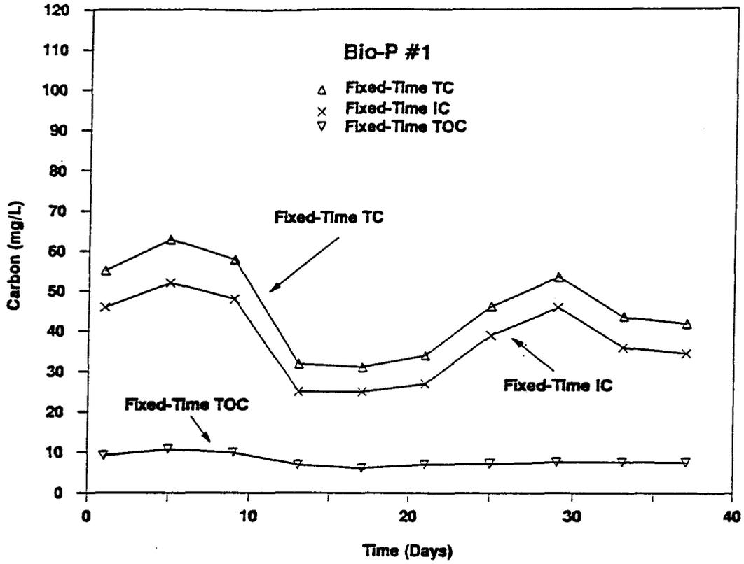
Figure 5.25 Carbon (TC, IC, TOC) Plots for FT RCTR: Bio-P#1
