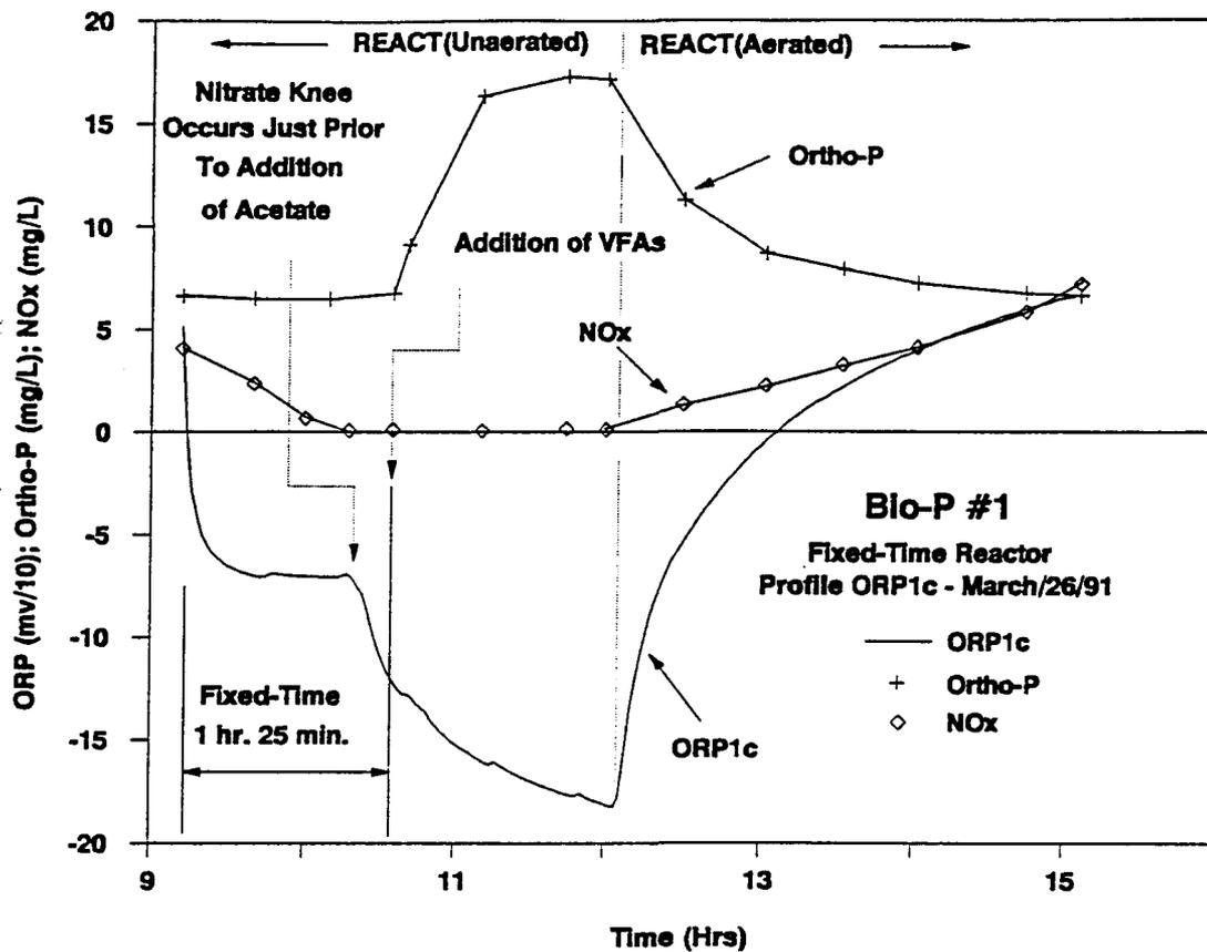
Figure 5.3 Fixed-Time Reactor Track Study: Bio-P#1
