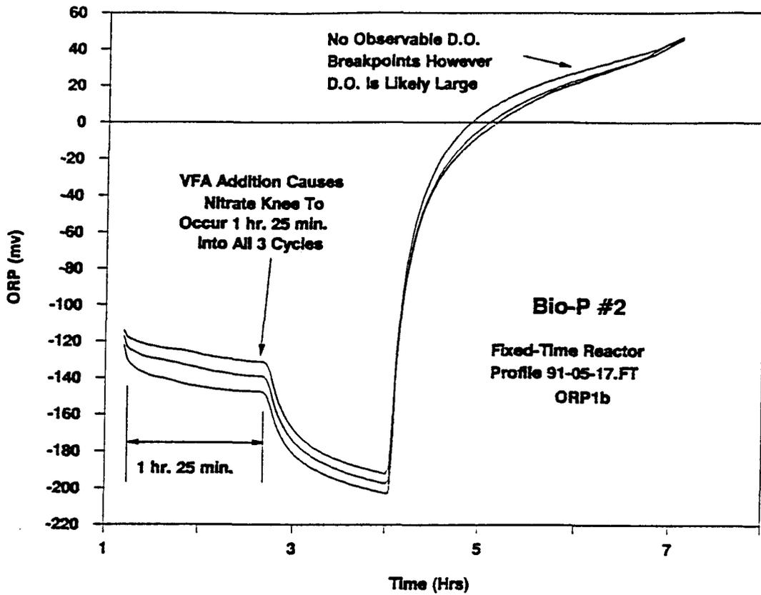
Figure 5.5 VFA-Caused Breakpoints in Fixed-Time Reactor
