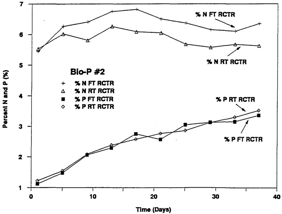
Figure 5.18 Reactor Plot of Percent N and P: Bio-P#2
