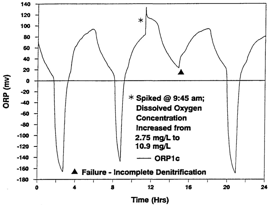
Figure 4.49 Spike of Hydrogen Peroxide to FT Reactor: AASD#2
