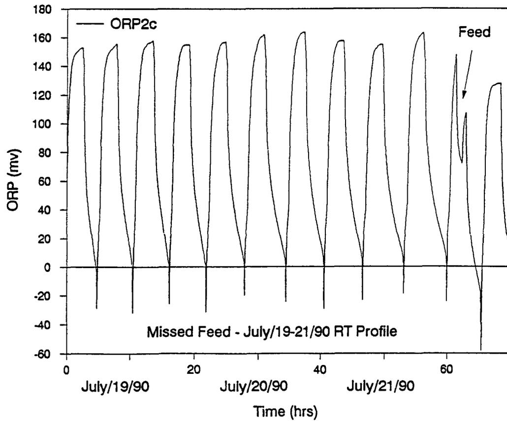
Figure 4.32 Real-Time Reactor Response to Missed Feed: AASD#1
