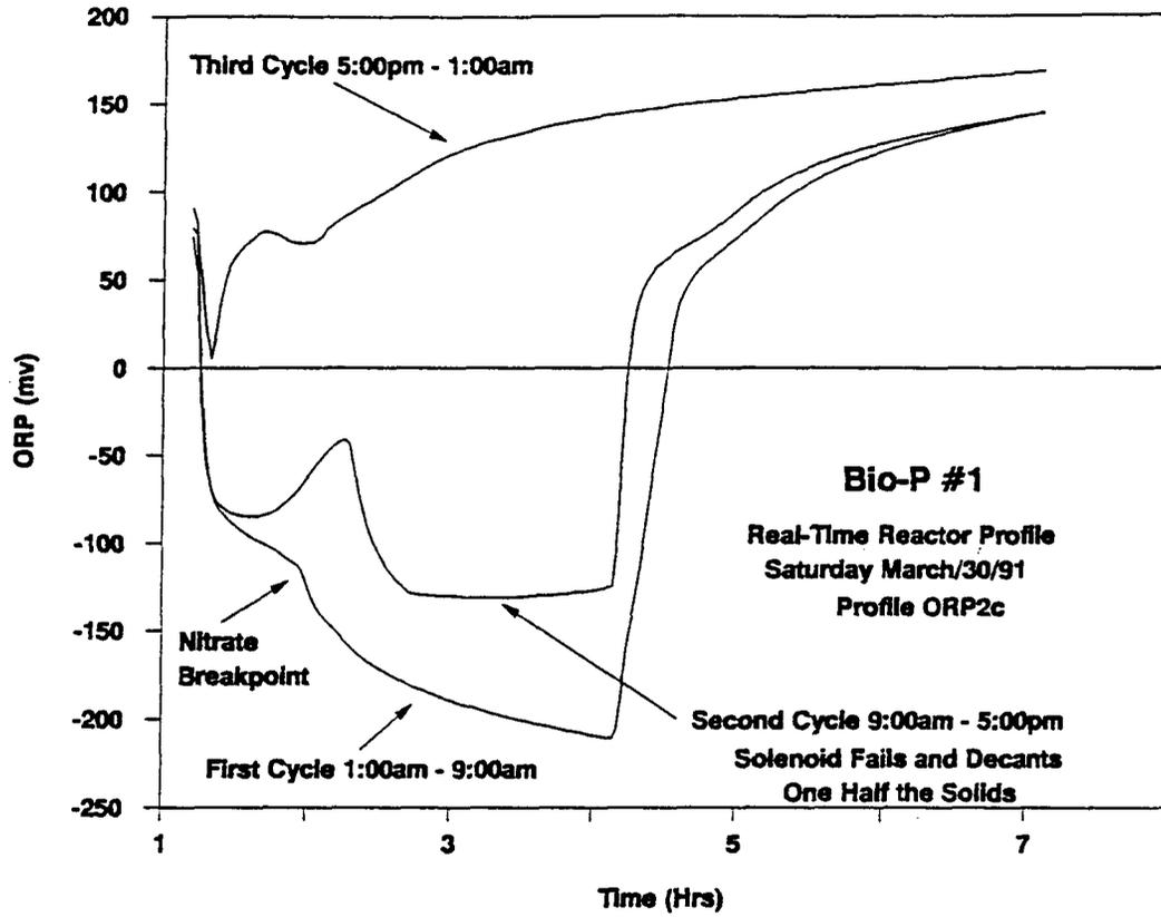
Figure 5.31 Disruption of Reactor Due to Solenoid Failure
