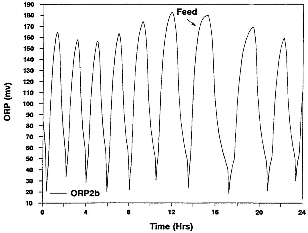
Figure 4.34 Real-Time ORP Profile Under AASD#2 Conditions
