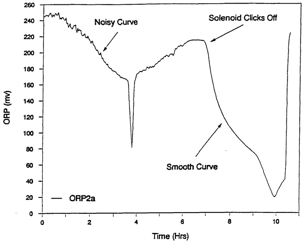
Figure 4.7 ORP Profile Affected by Intermittent Electrical Noise
