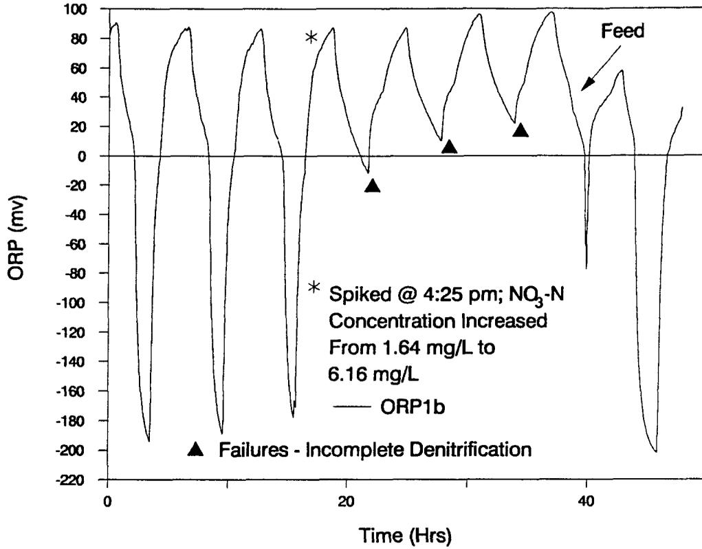
Figure 4.45 Spike of Sodium Nitrate to FT Reactor: AASD#2
