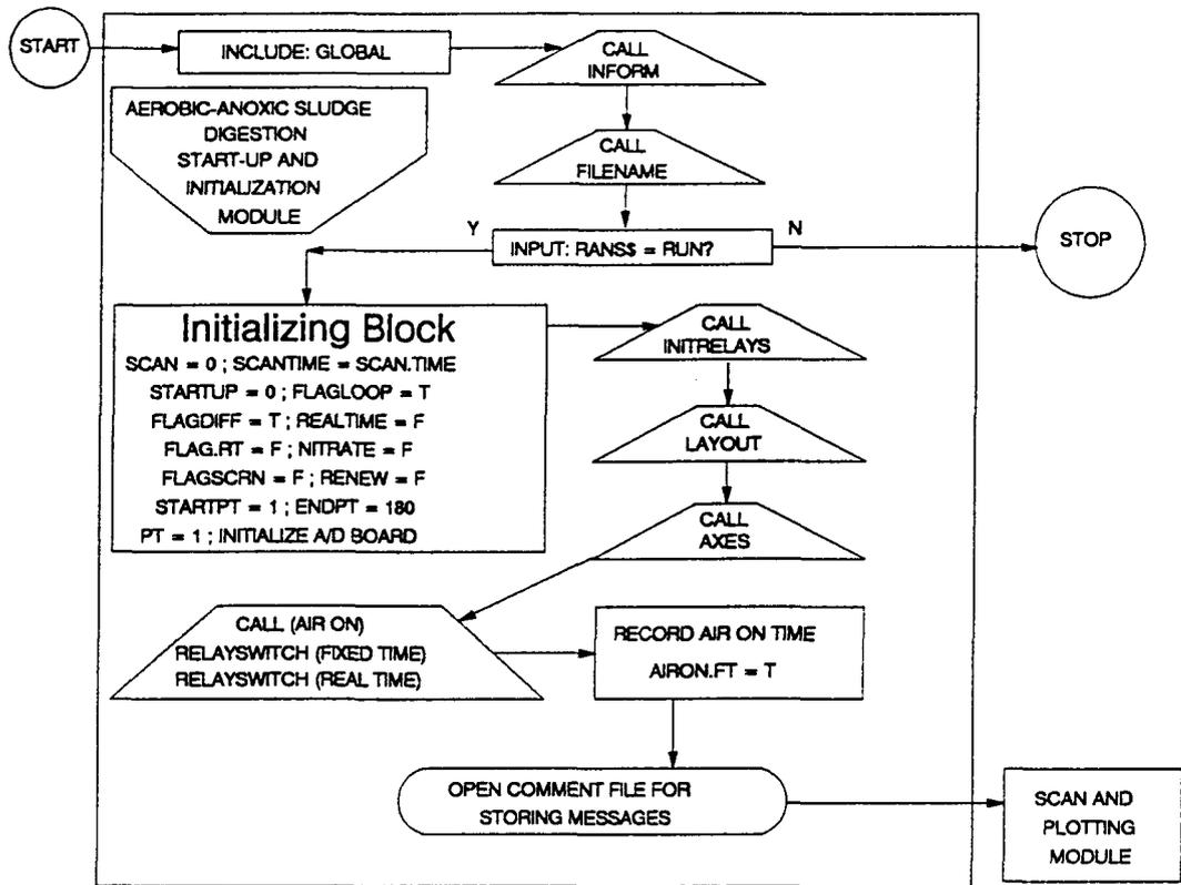
FIGURE C.1 AASD START-UP AND INITIALIZATION MODULE
