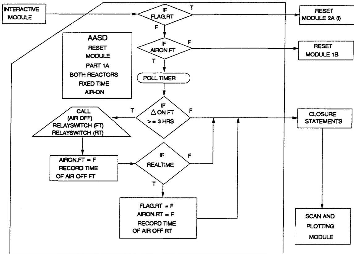
FIGURE C.4 AASD RESET MODULE - 1A - BOTH RCTRS FT - AIR ON
