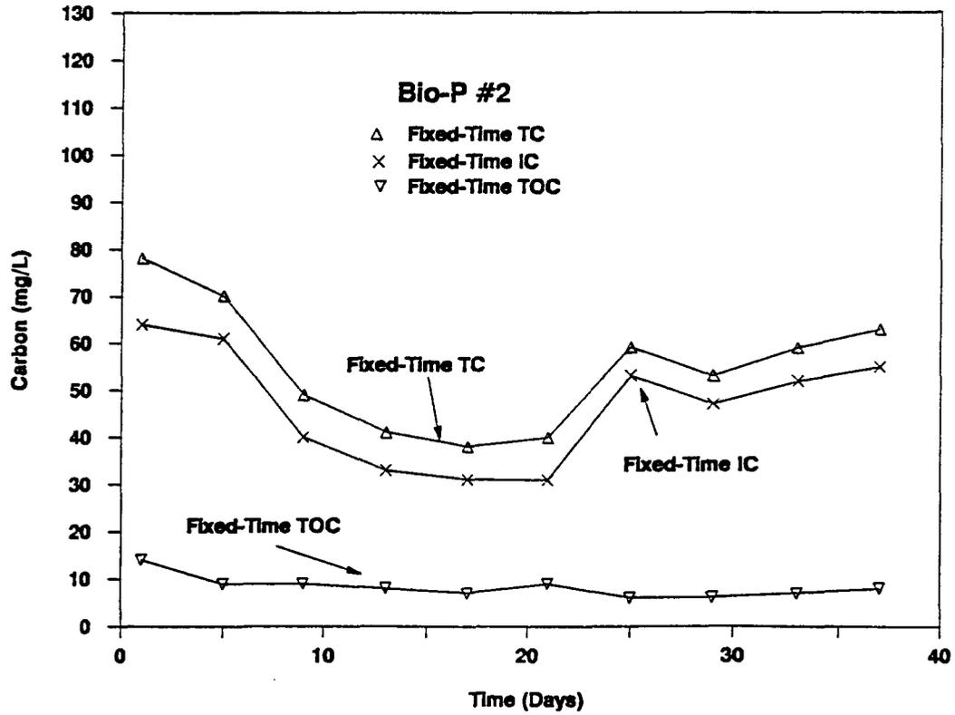
Figure 5.26 Carbon (TC, IC, TOC) Plots for FT RCTR: Bio-P#2
