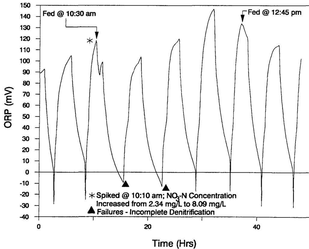
Figure 4.24 High Spike of Sodium Nitrate to RT Reactor: AASD#1
