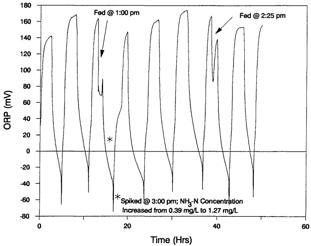
Figure 4.26 Low Spike of Ammonium Chloride to RT Reactor: AASD#1
