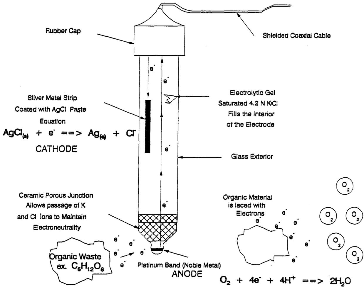
Figure 2.2 Diagram of ORP Electrode and Operation
