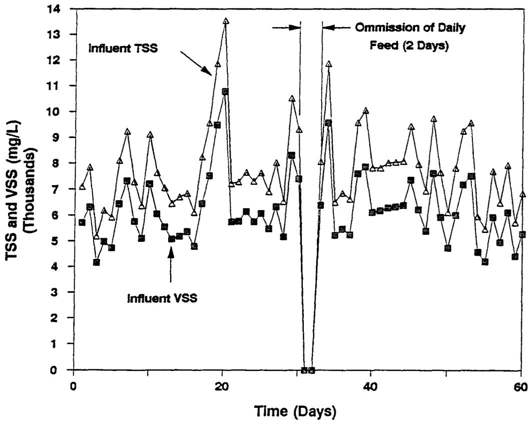
Figure 4.17 Parallel Plot: Feed Sludge AASD#1 TSS/VSS Ratio
