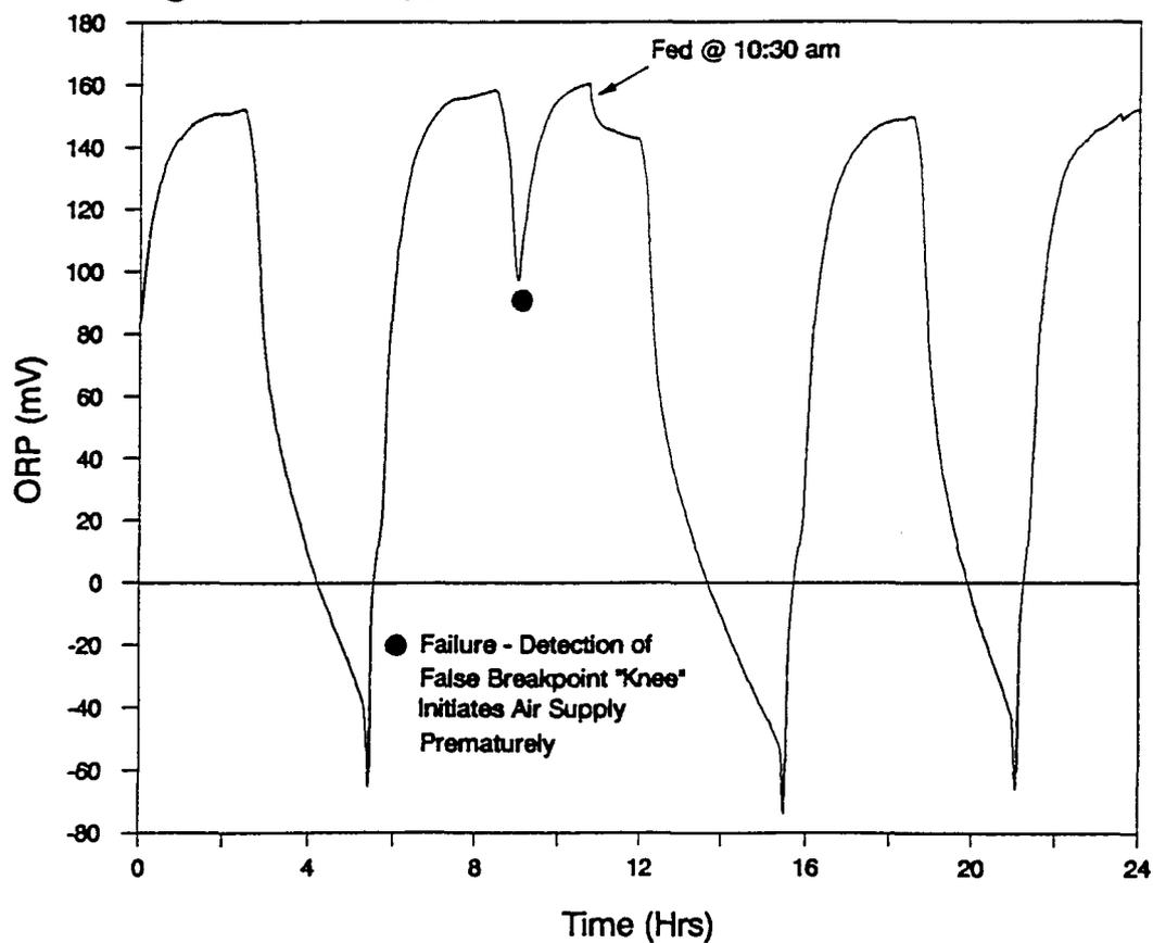
Figure 4.30 "False-Knee" Failure In Real-Time ORP Profile
