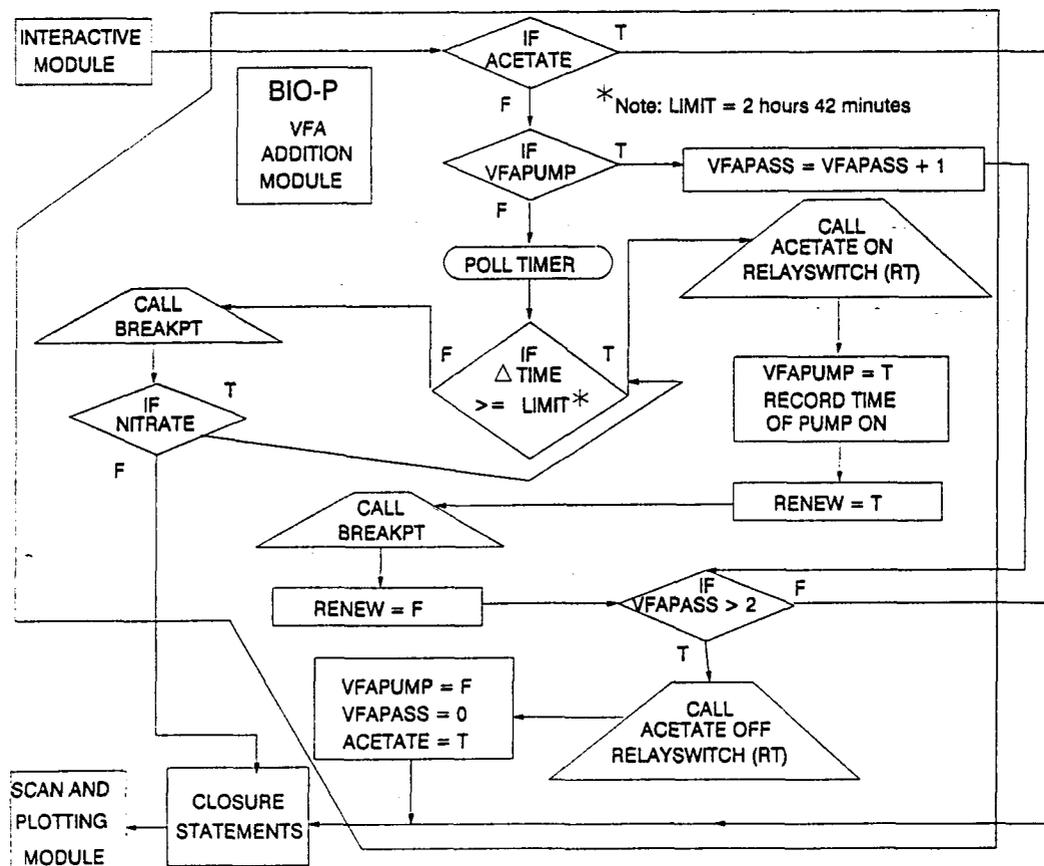
FIGURE C.15 BIO-P VFA ADDITION TO REAL-TIME REACTOR MODULE
