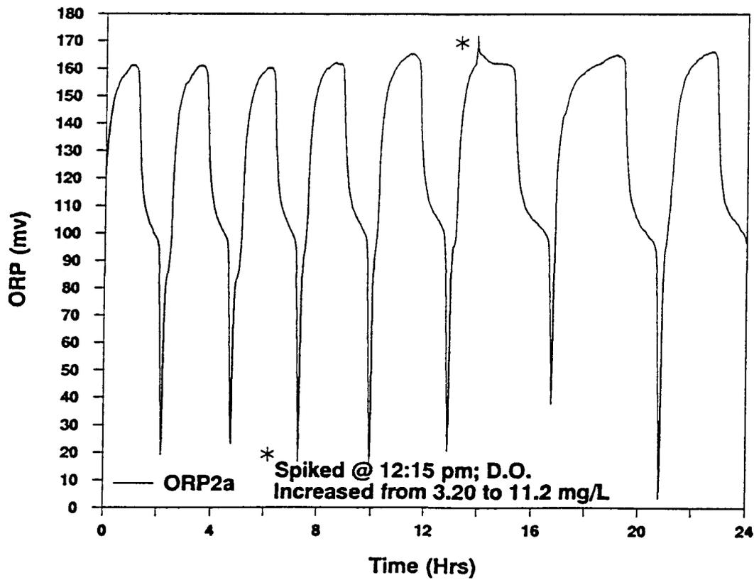
Figure 4.50 Spike of Hydrogen Peroxide to RT Reactor: AASD#2
