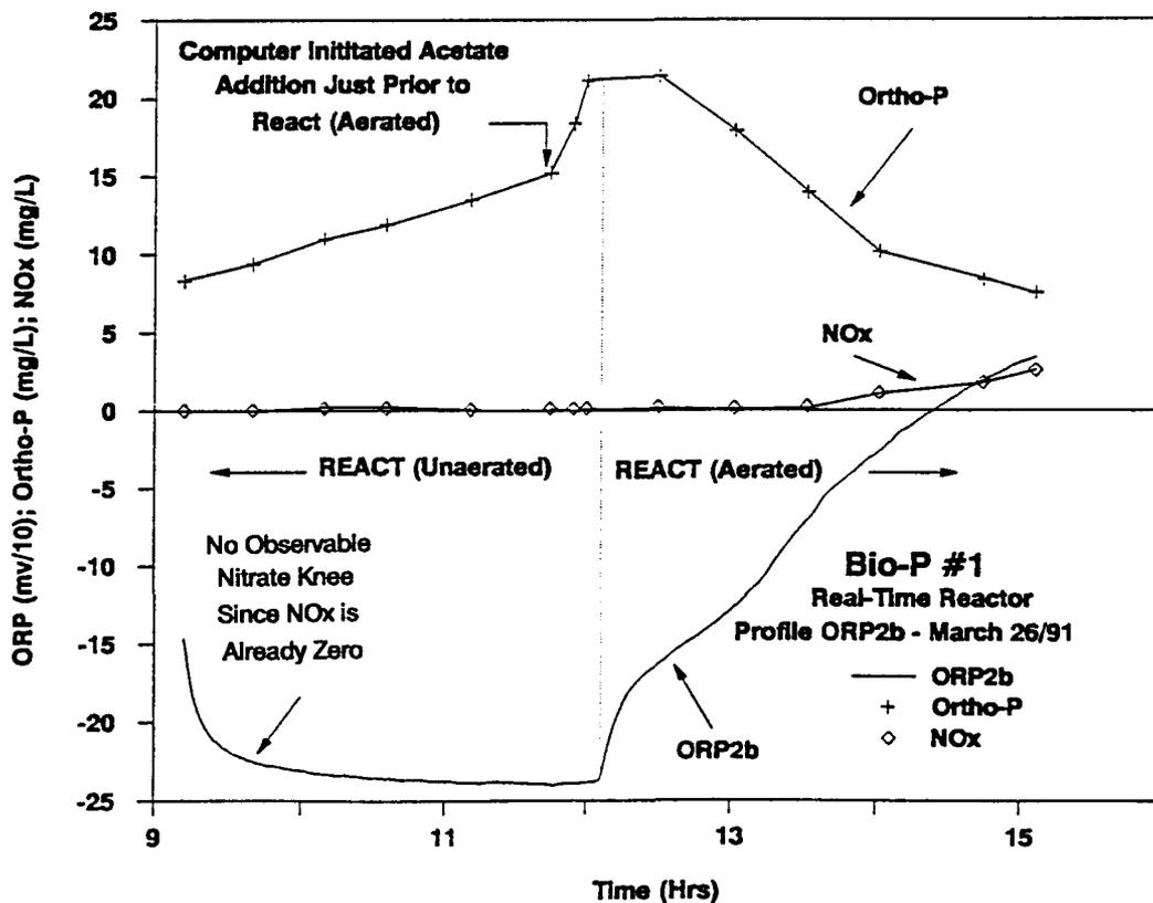
Figure 5.4 Real-Time Reactor Track Study: Bio-P#1
