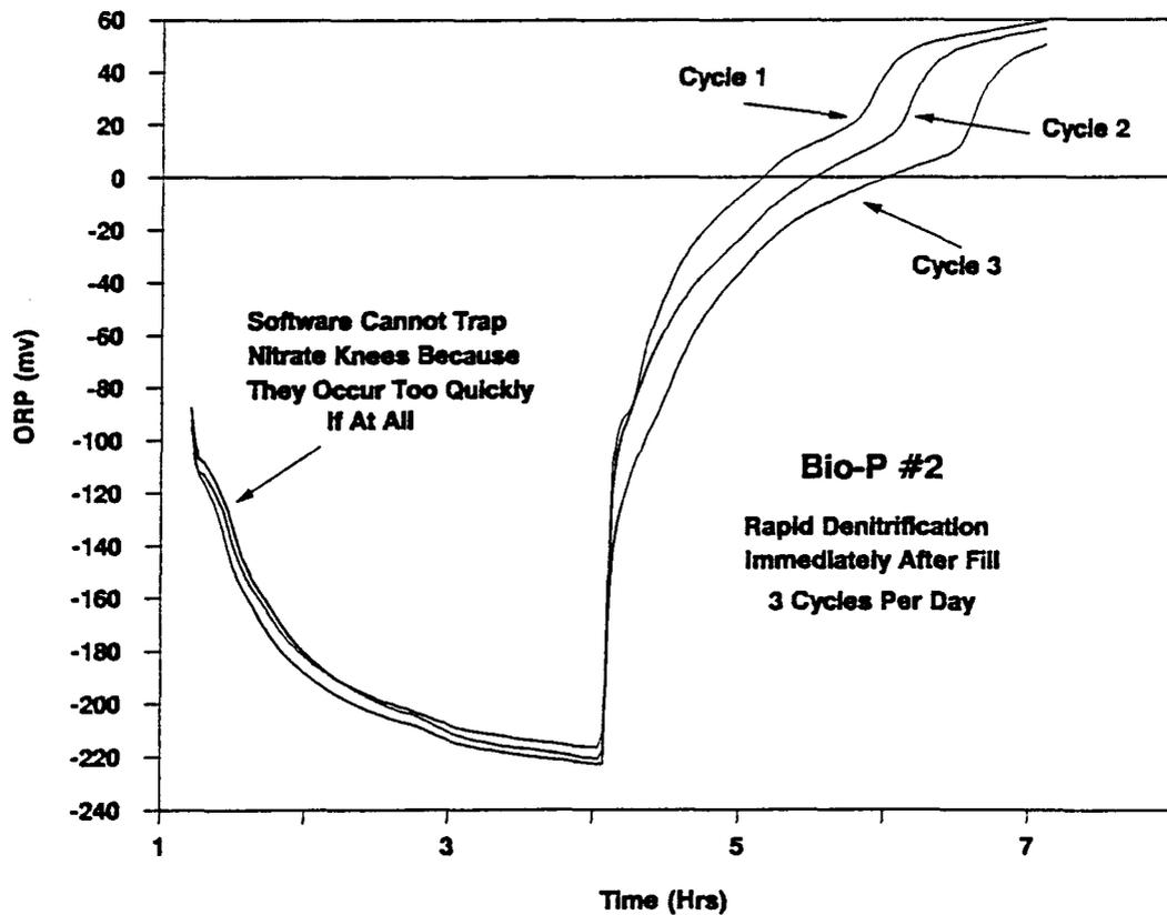
Figure 5.2 Software Failure Due to Rapid Denitrification
