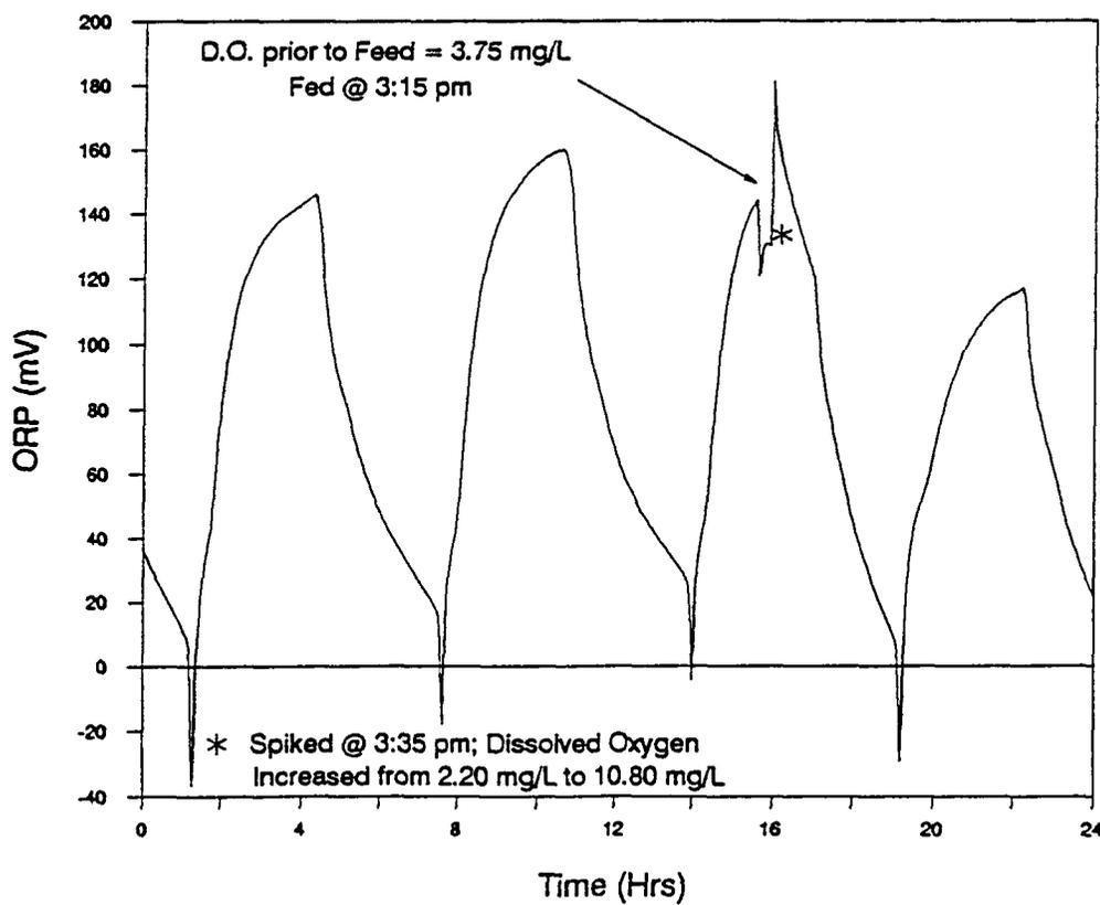
Figure 4.28 High Spike of Hydrogen Peroxide to RT Reactor: AASD#1
