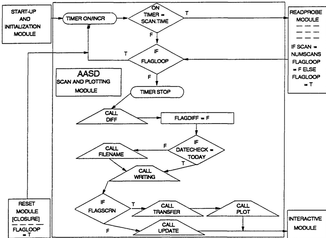
FIGURE C.2 AASD SCAN AND PLOTTING MODULE
