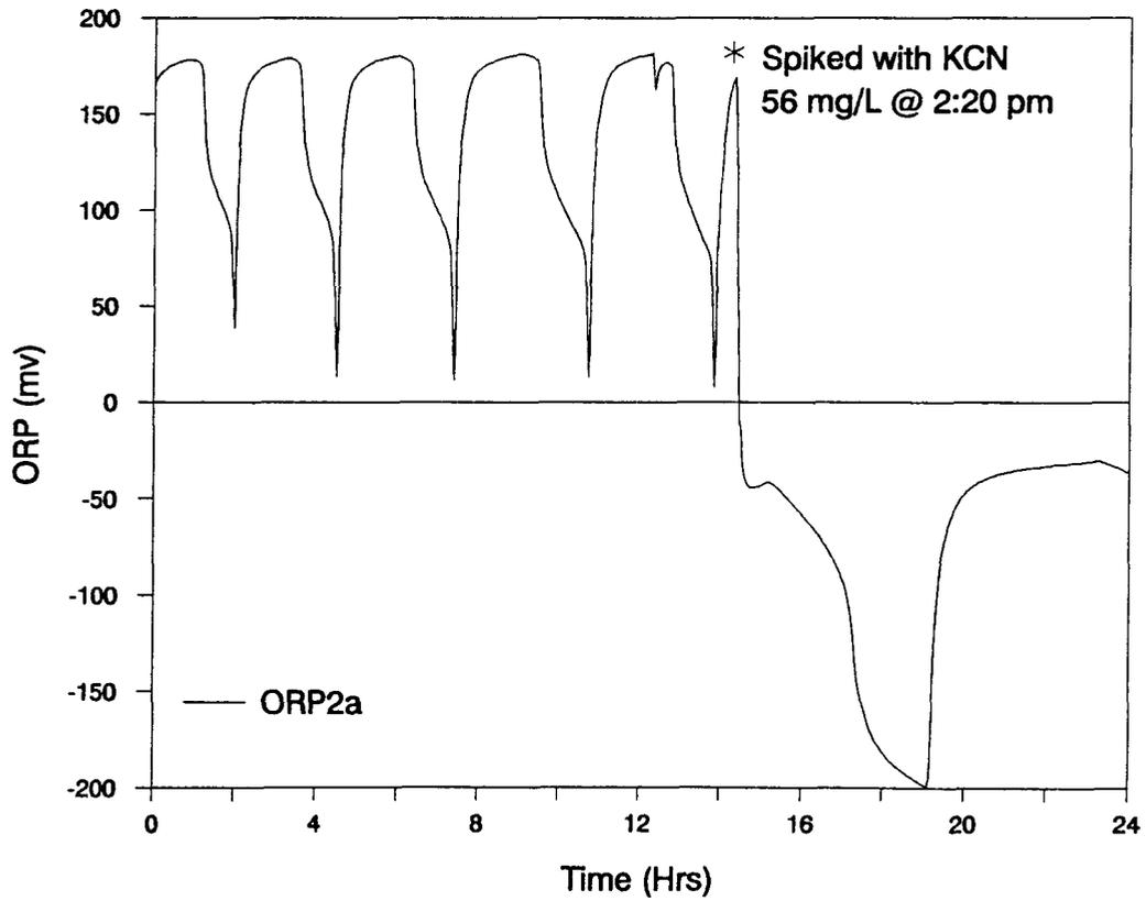
Figure 4.52 Spike of Potassium Cyanide to RT Reactor: AASD#2
