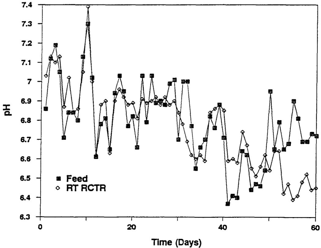
Figure 4.21 Real-Time Reactor: pH vs. Time for AASD<sup>#1</sup>
