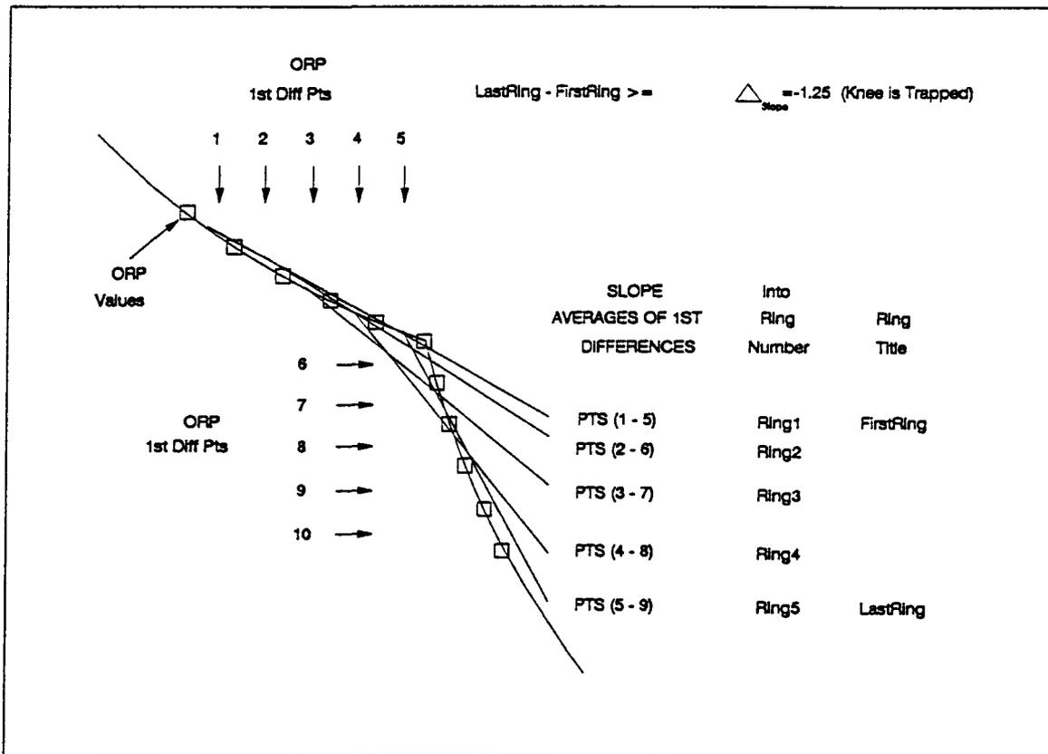
Figure 3.7 Illustration of BREAKPT Capture of Nitrate Knee
