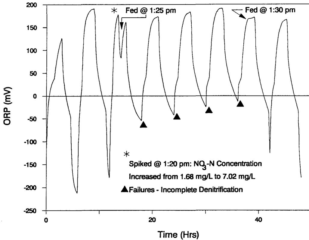
Figure 4.23 High Spike of Sodium Nitrate to FT Reactor: AASD#1
