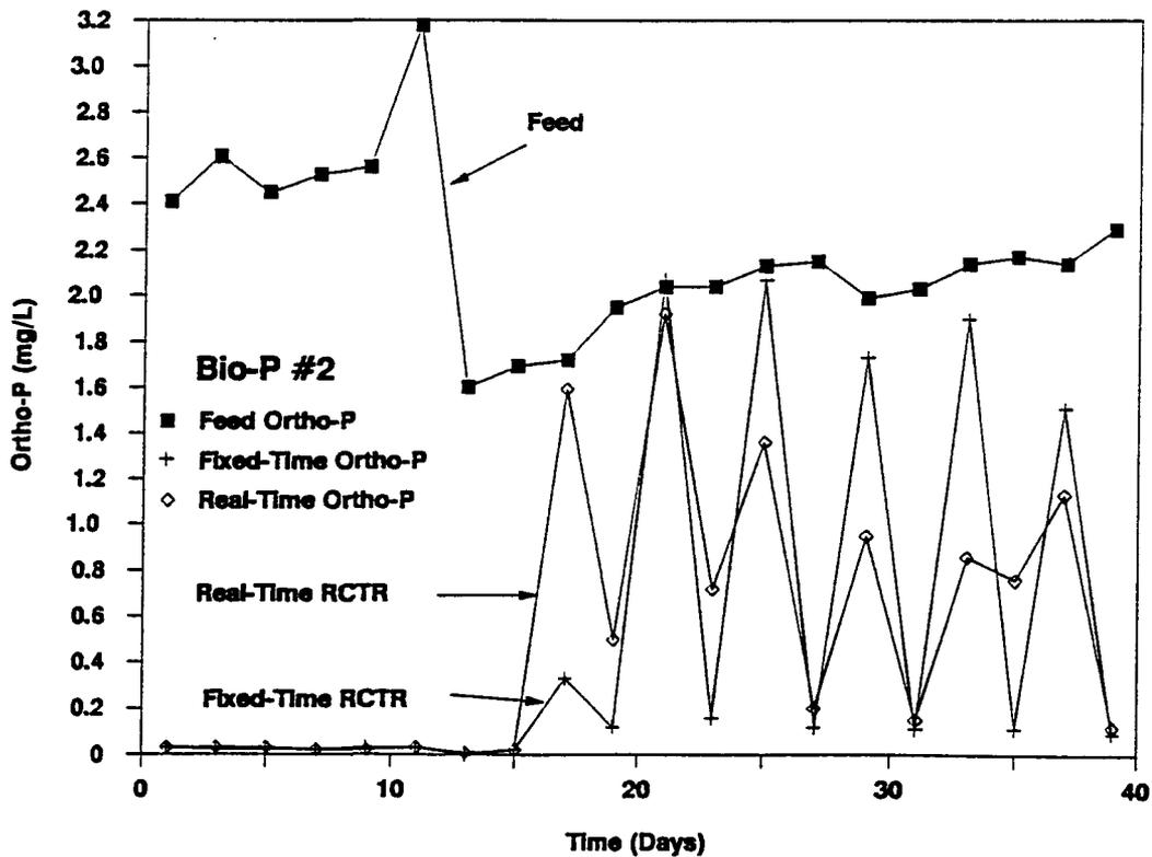
Figure 5.20 Track of Ortho-P Concentrations: Bio-P#2
