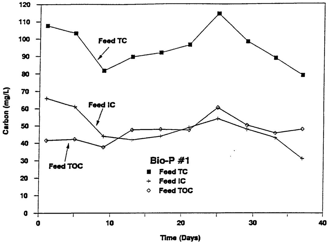
Figure 5.23 Carbon (TC, IC, TOC) Plots for Feed: Bio-P#1
