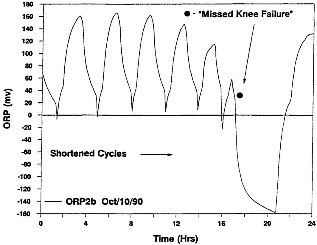
Figure 4.37 "Missed-Knee" Failure in Real-Time ORP Profile
