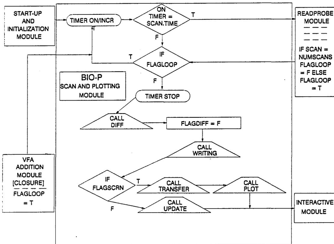
FIGURE C.13 BIO-P SCAN AND PLOTTING MODULE
