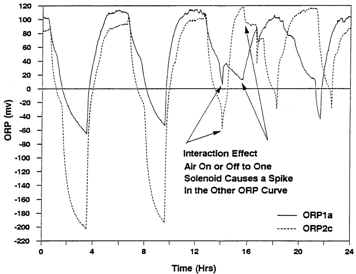
Figure 4.6 Reactor Interaction Effects Due to Improper Grounding
