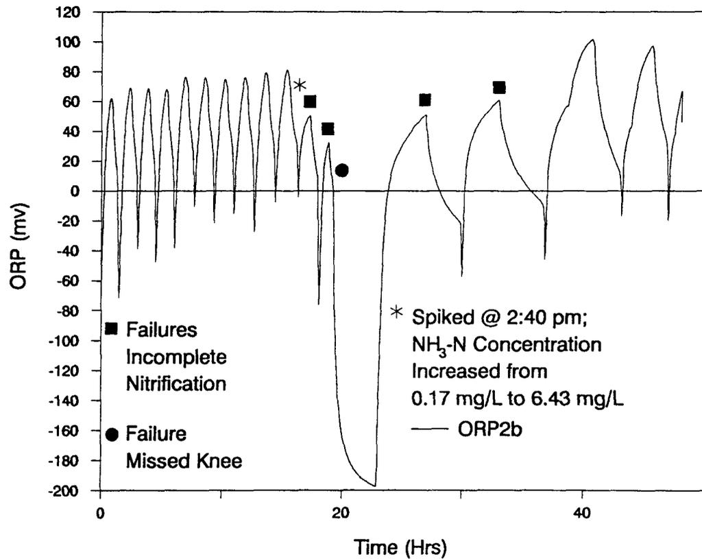
Figure 4.48 Spike of Ammonium Chloride to RT Reactor: AASD#2
