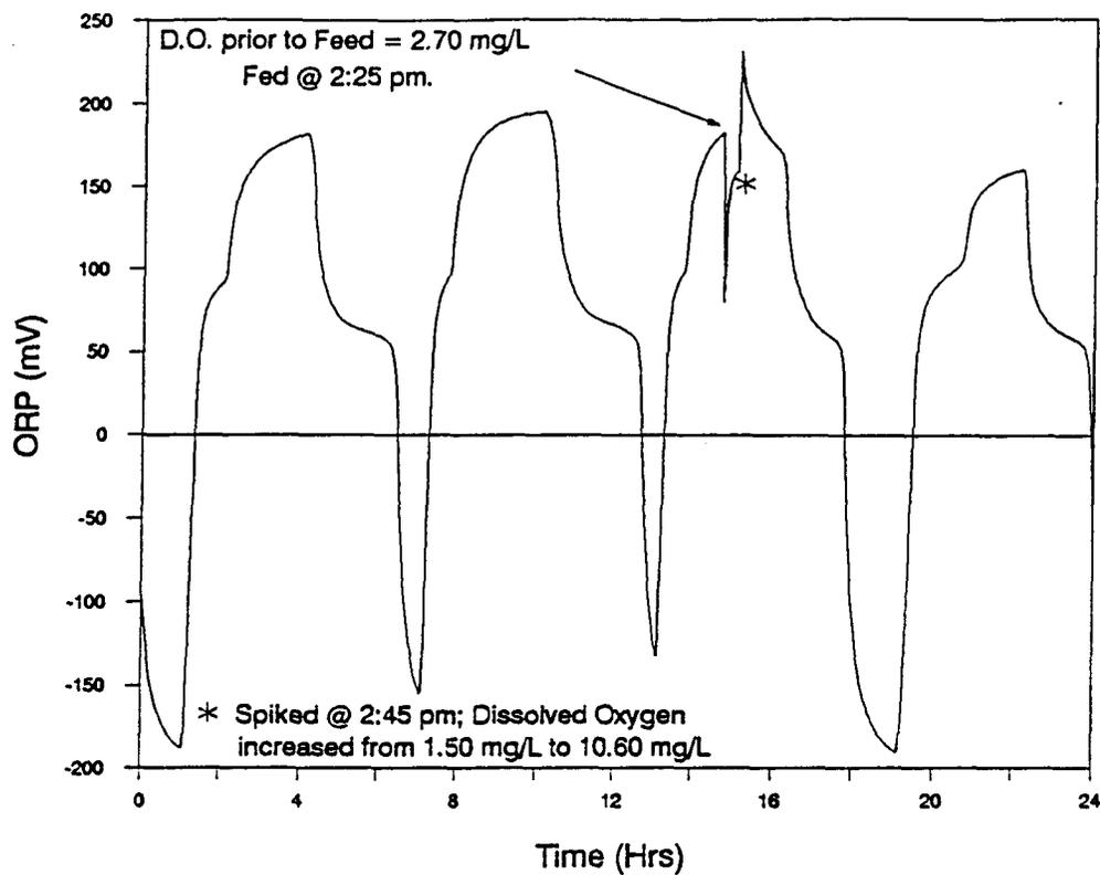
Figure 4.27 High Spike of Hydrogen Peroxide to FT Reactor: AASD#1
