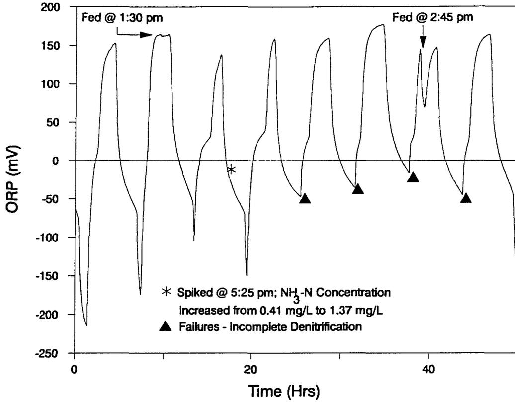
Figure 4.25 Low Spike of Ammonium Chloride to FT Reactor: AASD#1
