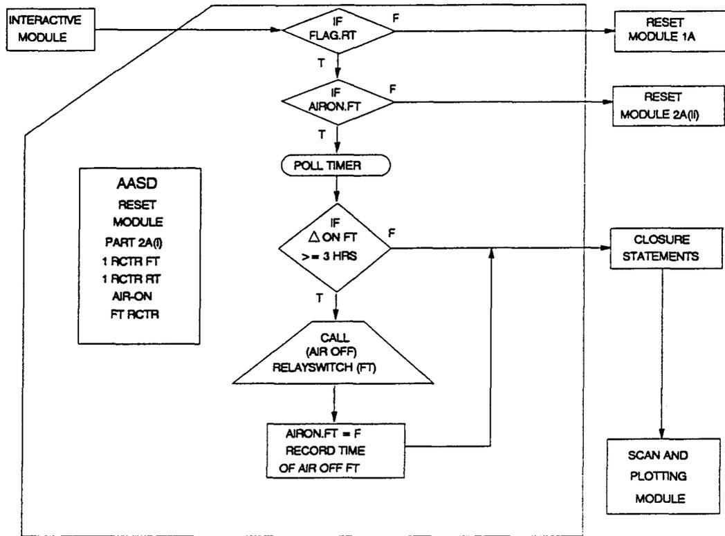
FIGURE C.6 AASD RESET MODULE - 2A(i) - RT CONTROL - AIR ON FT
