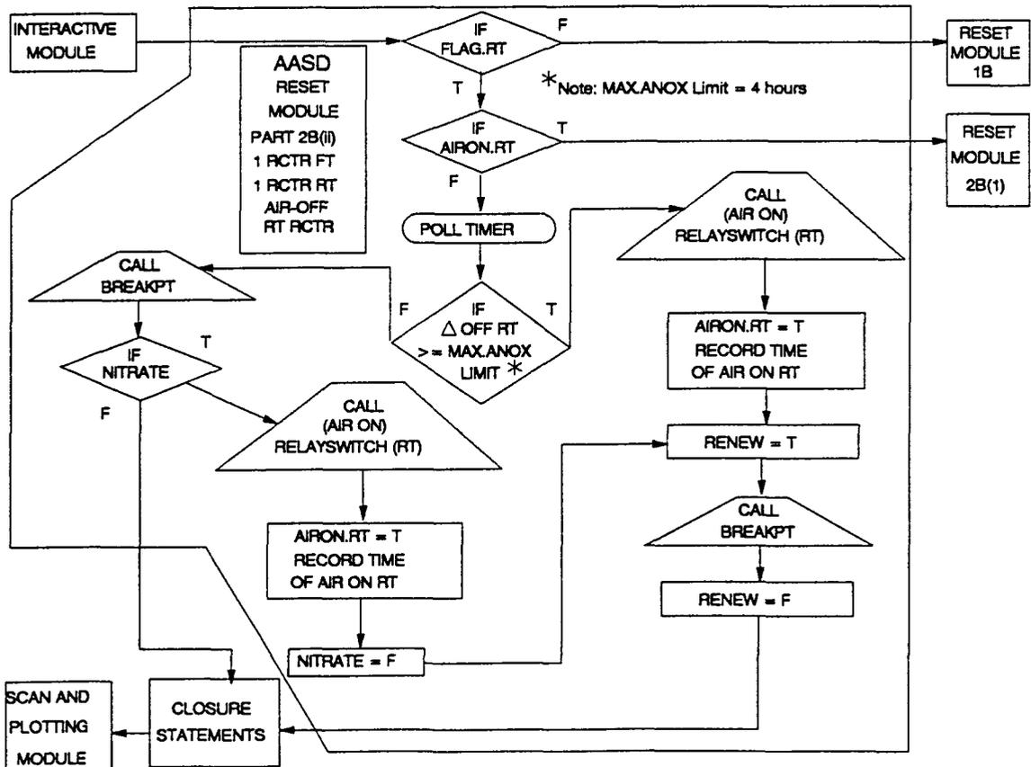
FIGURE C.9 AASD RESET MODULE - 2B(ii) - RT CONTROL - AIR OFF RT
