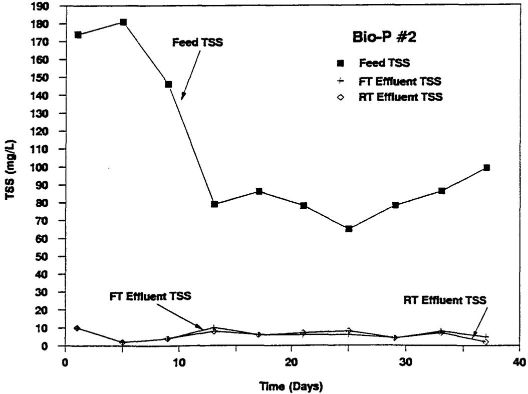
Figure 5.14 Variation in Feed and Effluent TSS: Bio-P#2
