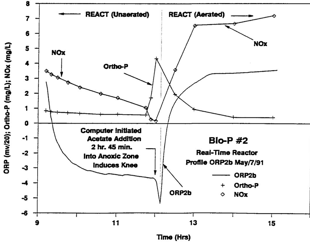
Figure 5.8 Real-Time Reactor Track Study: Bio-P#2
