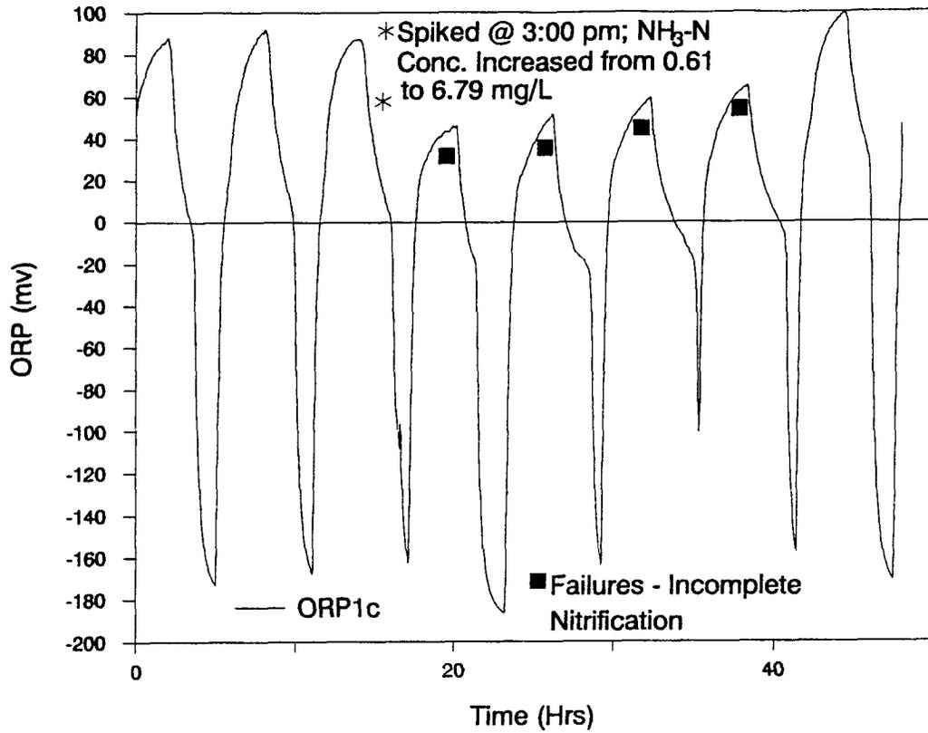
Figure 4.47 Spike of Ammonium Chloride to FT Reactor: AASD#2
