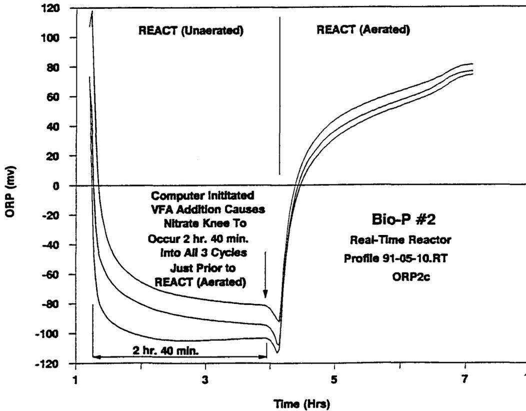
Figure 5.6 VFA-Caused Breakpoints in Real-Time Reactor
