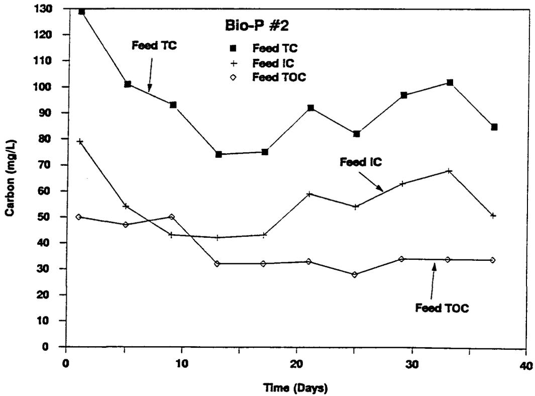
Figure 5.24 Carbon (TC, IC, TOC) Plots for Feed: Bio-P#2
