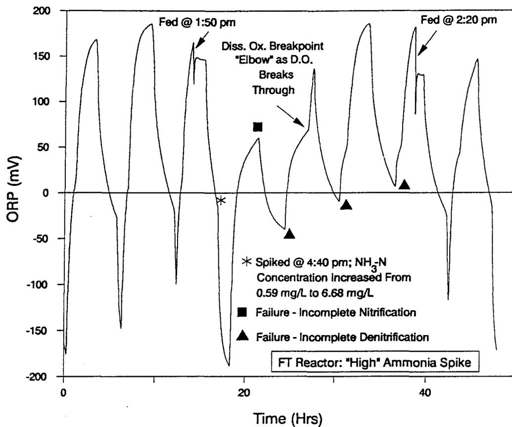
Figure 4.29 Typical "Incomplete Nitrification Failure"
