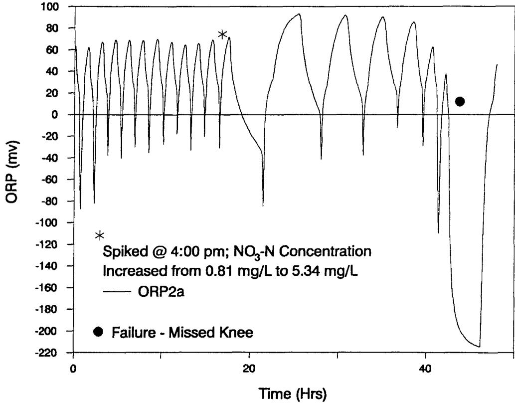
Figure 4.46 Spike of Sodium Nitrate to RT Reactor: AASD#2
