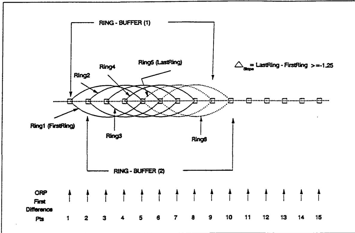
Figure 3.6 Illustration of Linear Ring-Buffer Concept
