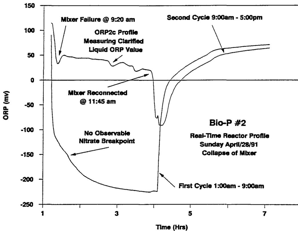
Figure 5.32 Disruption of Reactor Due to Mixer Failure
