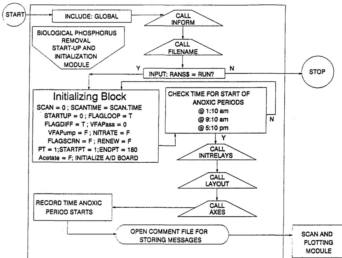
FIGURE C.12 BIO-P START-UP AND INITIALIZATION MODULE
