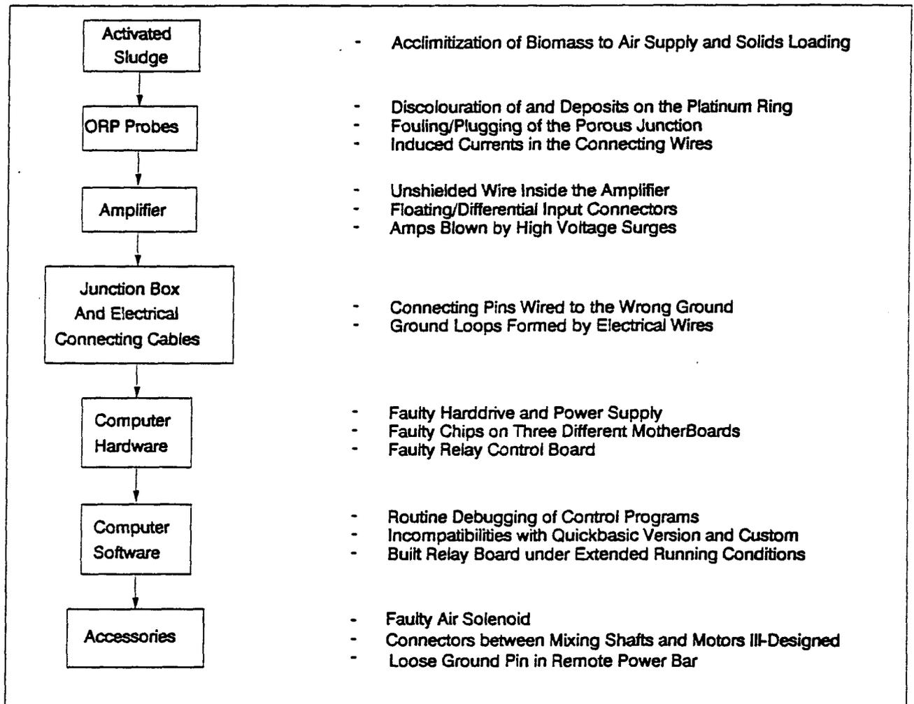
Figure 4.5 Linear Diagram of Components Identifying Problem Areas
