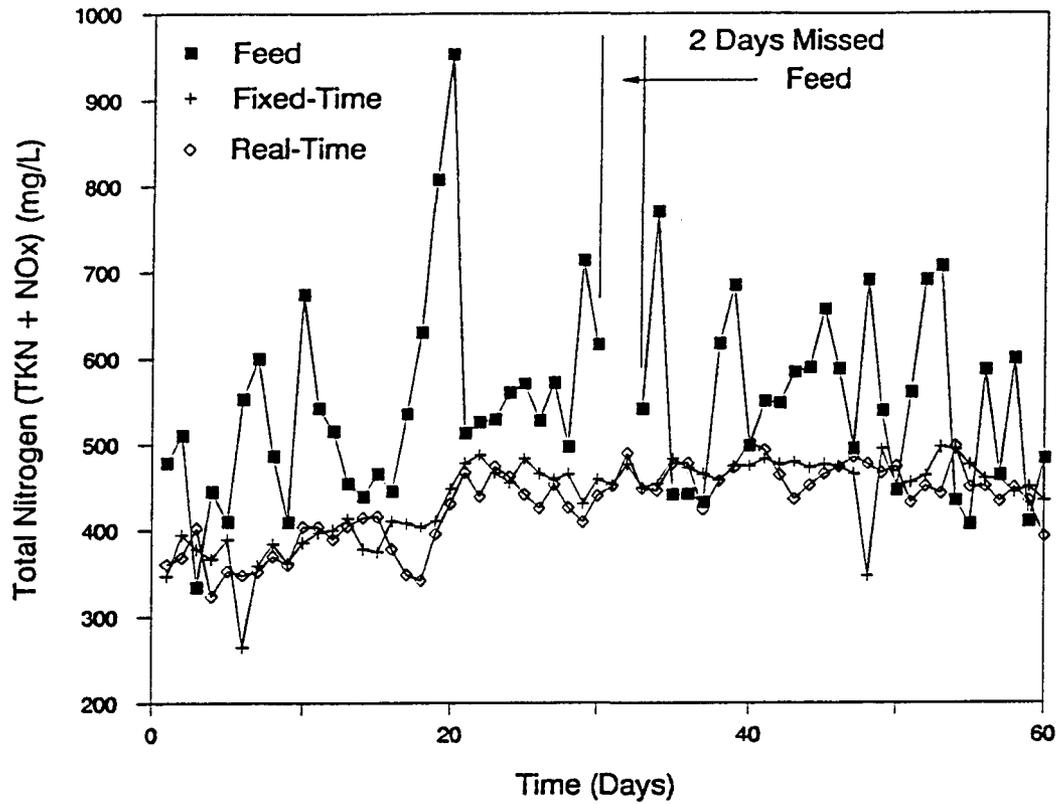
Figure 4.18 Fluctuations in Total Nitrogen Content: AASD#1
