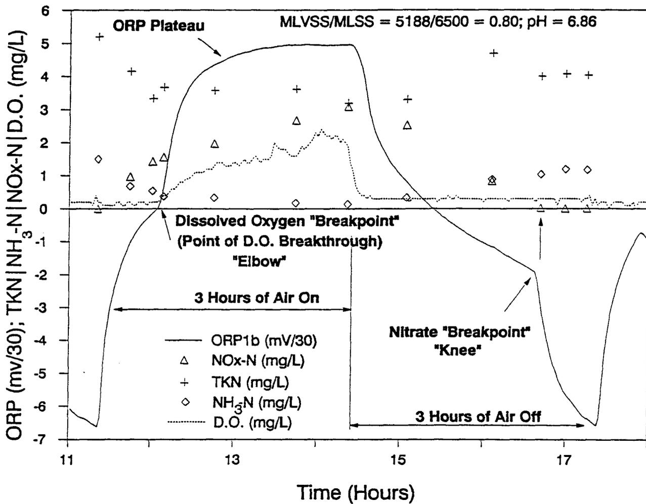
Figure 4.1 Fixed-Time ORP Profile Under AASD Conditions
