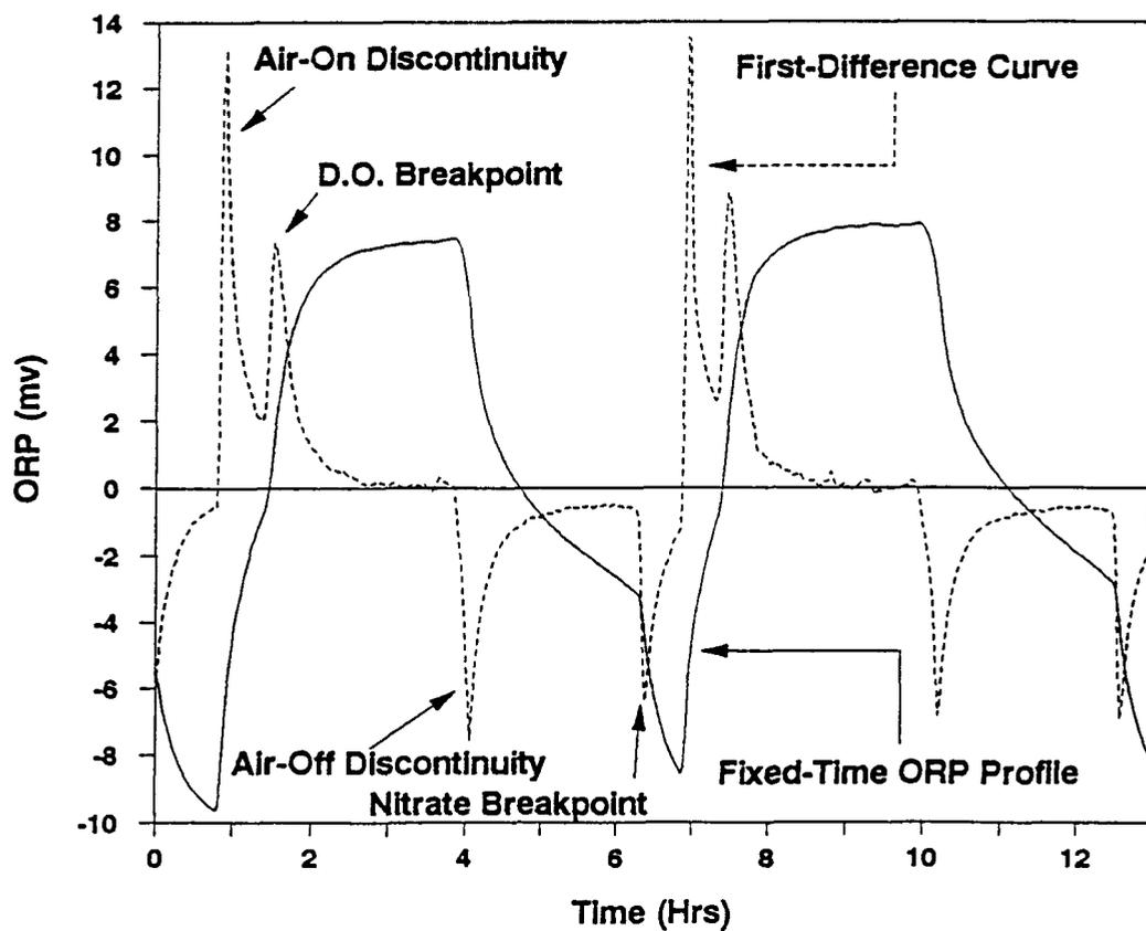
Figure 4.4 Overlay of First-Difference and ORP-Time Profiles
