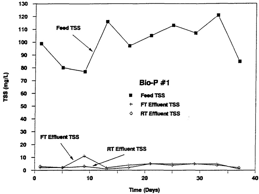
Figure 5.13 Variation in Feed and Effluent TSS: Bio-P#1
