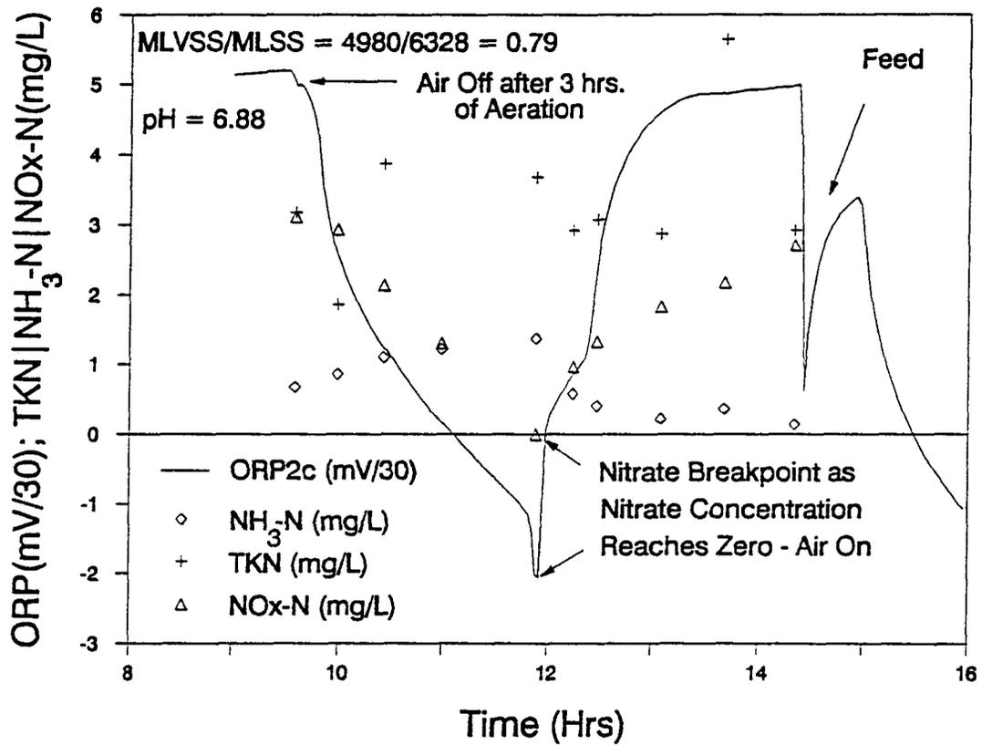
Figure 4.2 Real-Time ORP Profile Under AASD\*1 Conditions
