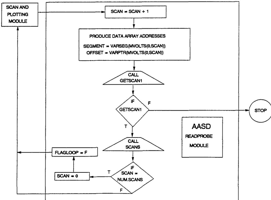
FIGURE C.11 AASD READPROBE MODULE
