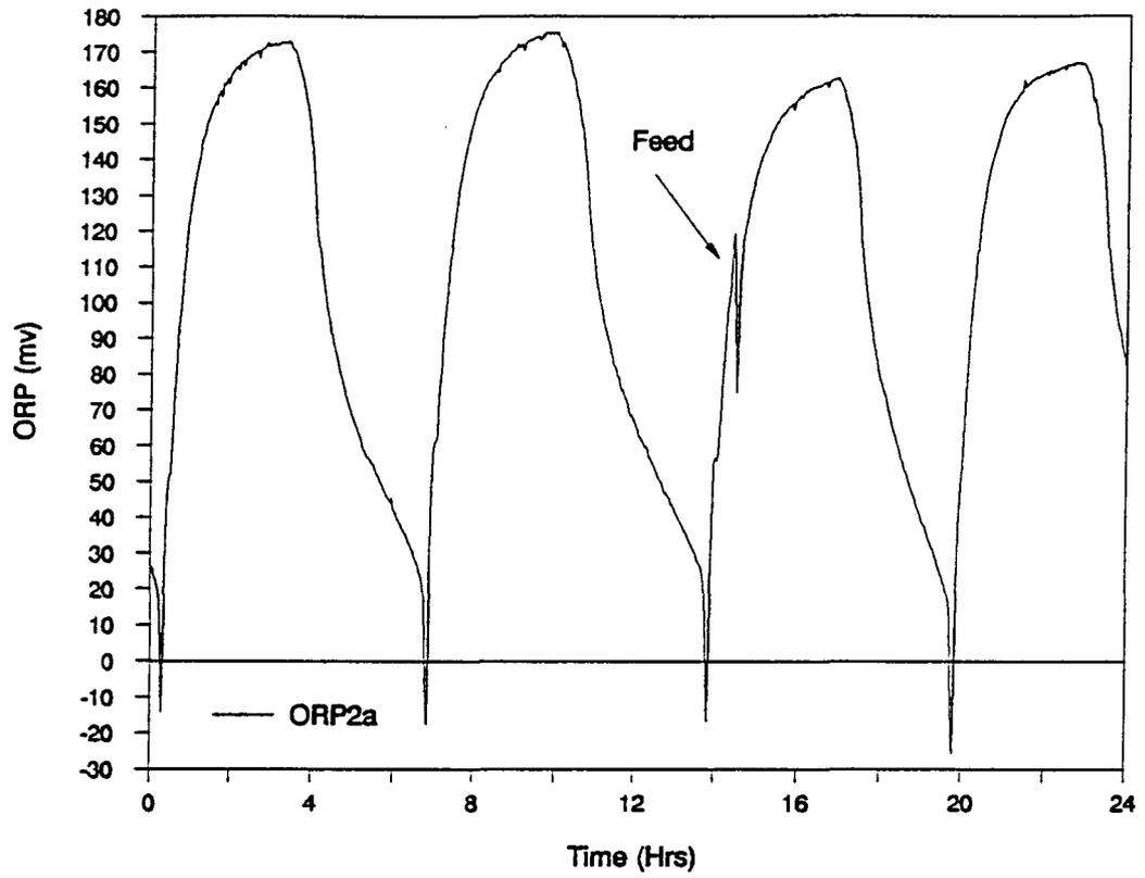
Figure 4.12 Temporal Reproducibility of ORP Curves in RT Reactor
