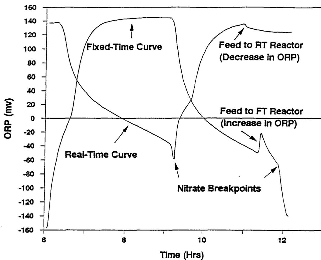
Figure 4.3 Effect of Relatively Fresh Feed on Reactor ORP Curves
