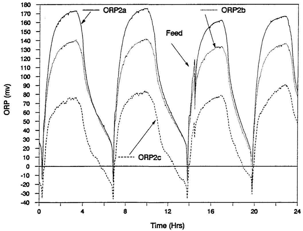
Figure 4.13 Spatial Reproducibility of 3 ORP Electrodes in Same Reactor
