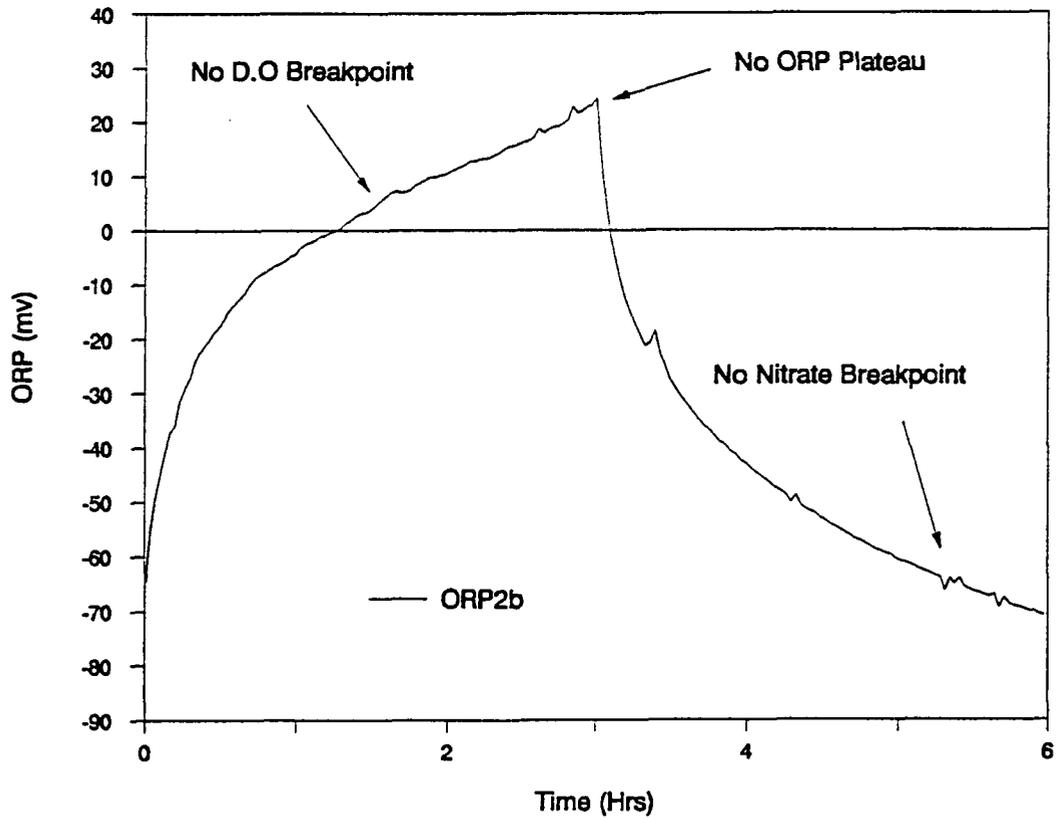
Figure 4.10 Unusual Response Pattern: No Diss. Oxygen Breakpoint
