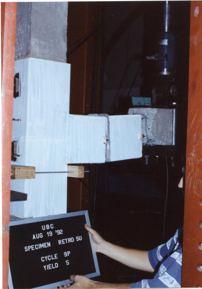
c) Hinge Formation During Negative Loading
