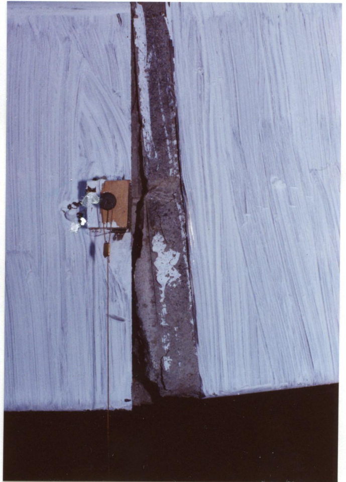
b) Hinge Formation During Positive Loading
