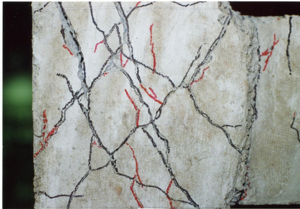
b) Shear Cracking in Joint Area
