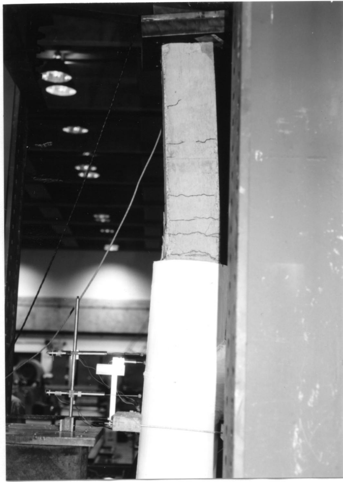
c) Column Hinge Formation During Negative Loading
