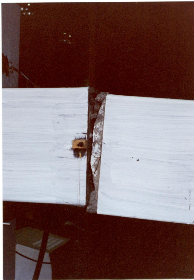
c) Hinge Formation During Negative Loading
