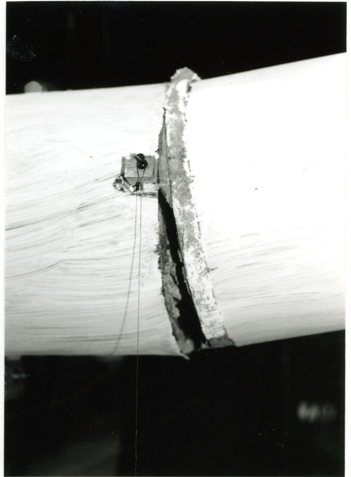
b) Hinge Formation During Positive Loading
