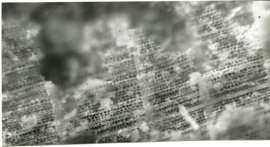
Figure 5.13: 'Brash' failure surface photographed in microscope (40x).
