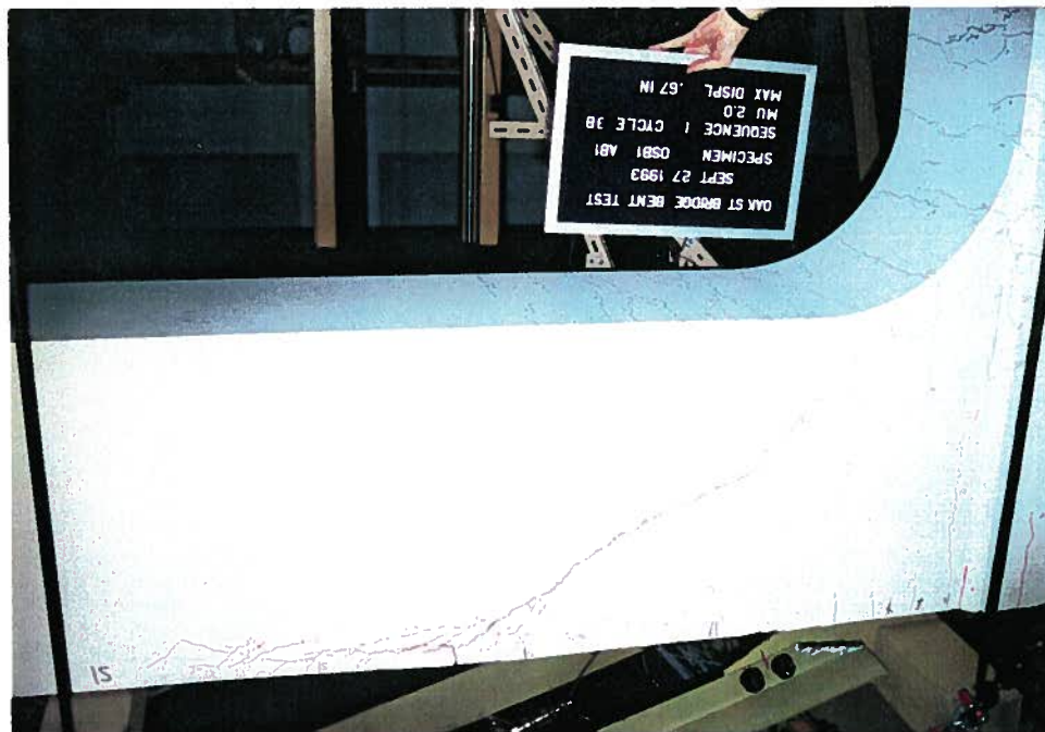
Fig. 6.17 Cap beam cracking Specimen OSB1
