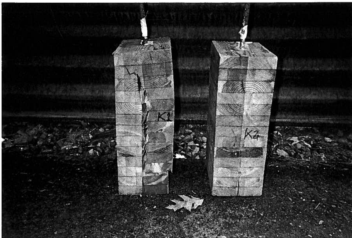
Fig.2.13 Photo of the specimens K2 (Failure Mode II) and K1 (Failure Mode III). Note that the top surface of the specimen K1 is not split.
