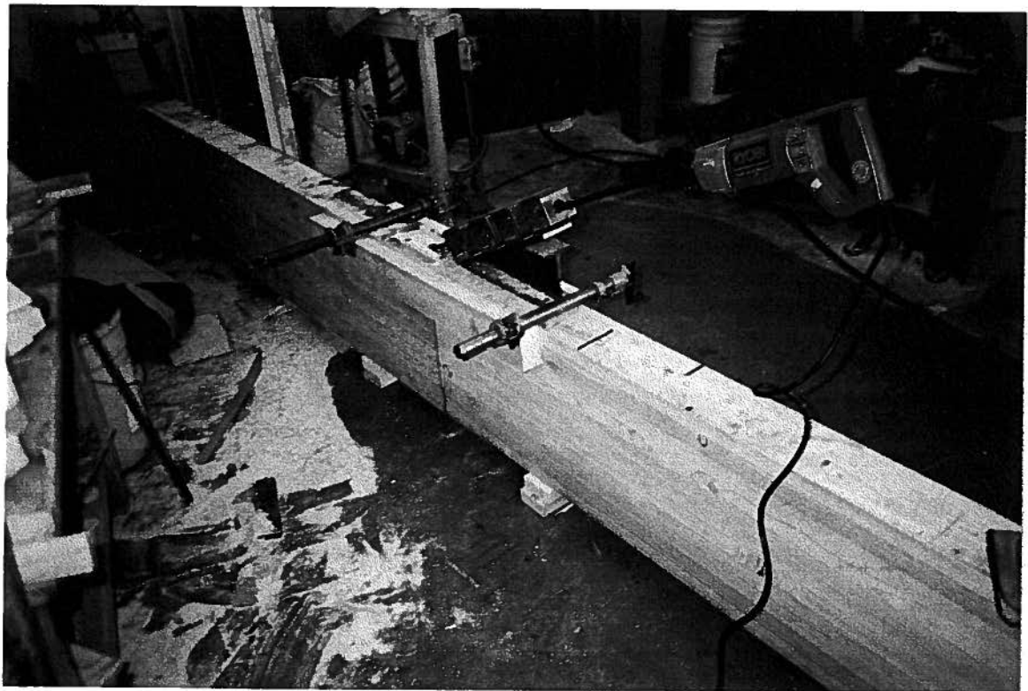
Fig.4.24 Drilling inclined holes.
