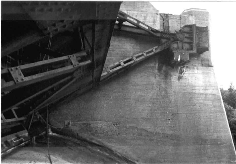
PHOTOGRAPH 7 Sensors located on west side of pier at node 16. RUSKIN DAM AMBIENT VIBRATION FIELD TEST, LOW RESERVOIR, 30 APRIL 94
