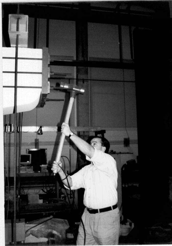
Figure 3.8 Longitudinal impact applied with the instrumented hammer
