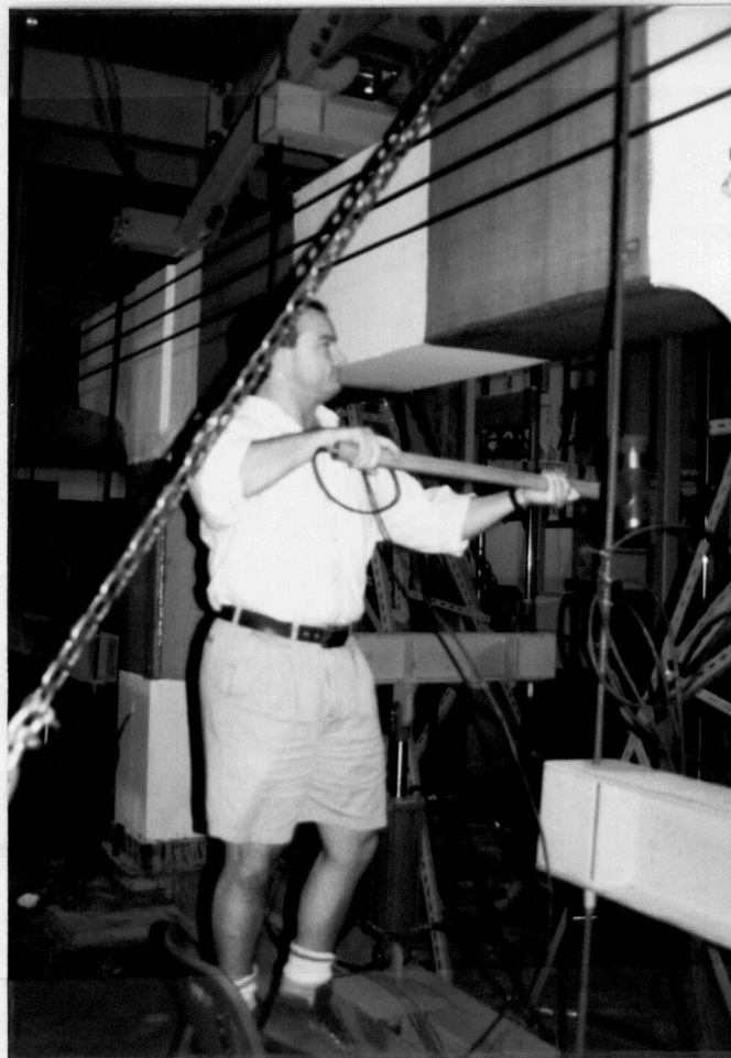
Figure A.5 Vertical impact applied with the instrumented hammer
