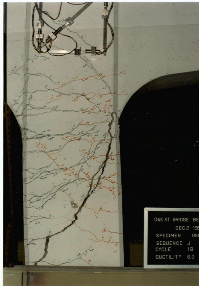
Figure A.8 View of specimen OSB2 at failure (north column, east side)
