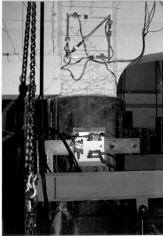
Figure 3.6 Installation device for accelerometers of OSB3 and OSB4
