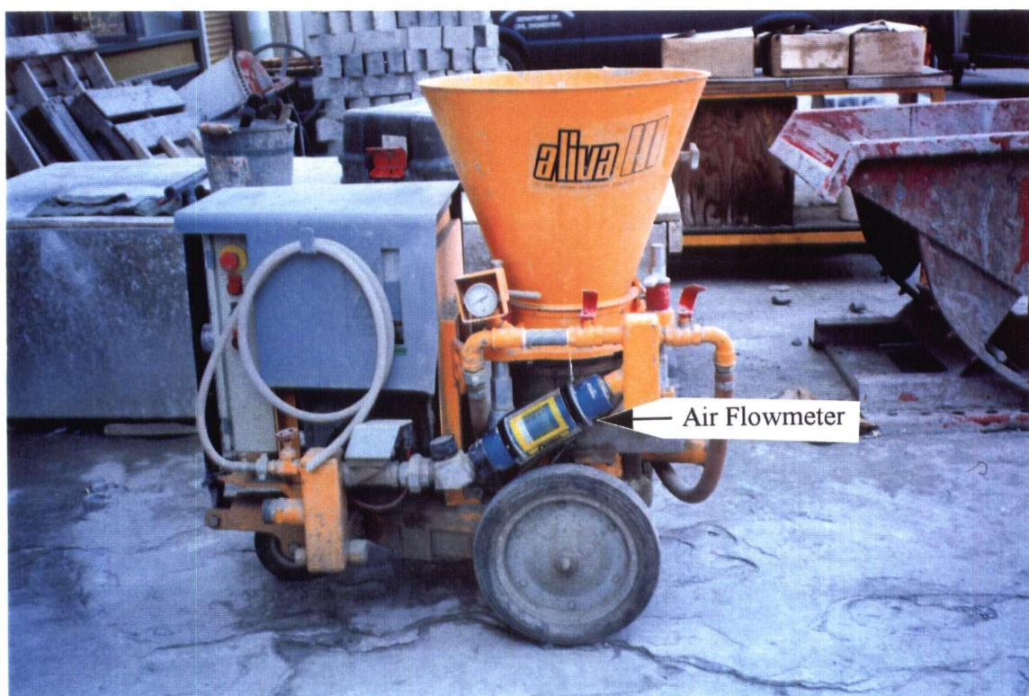
Figure B6 - Air flowmeter installed at the shotcrete machine's compressed air intake.
