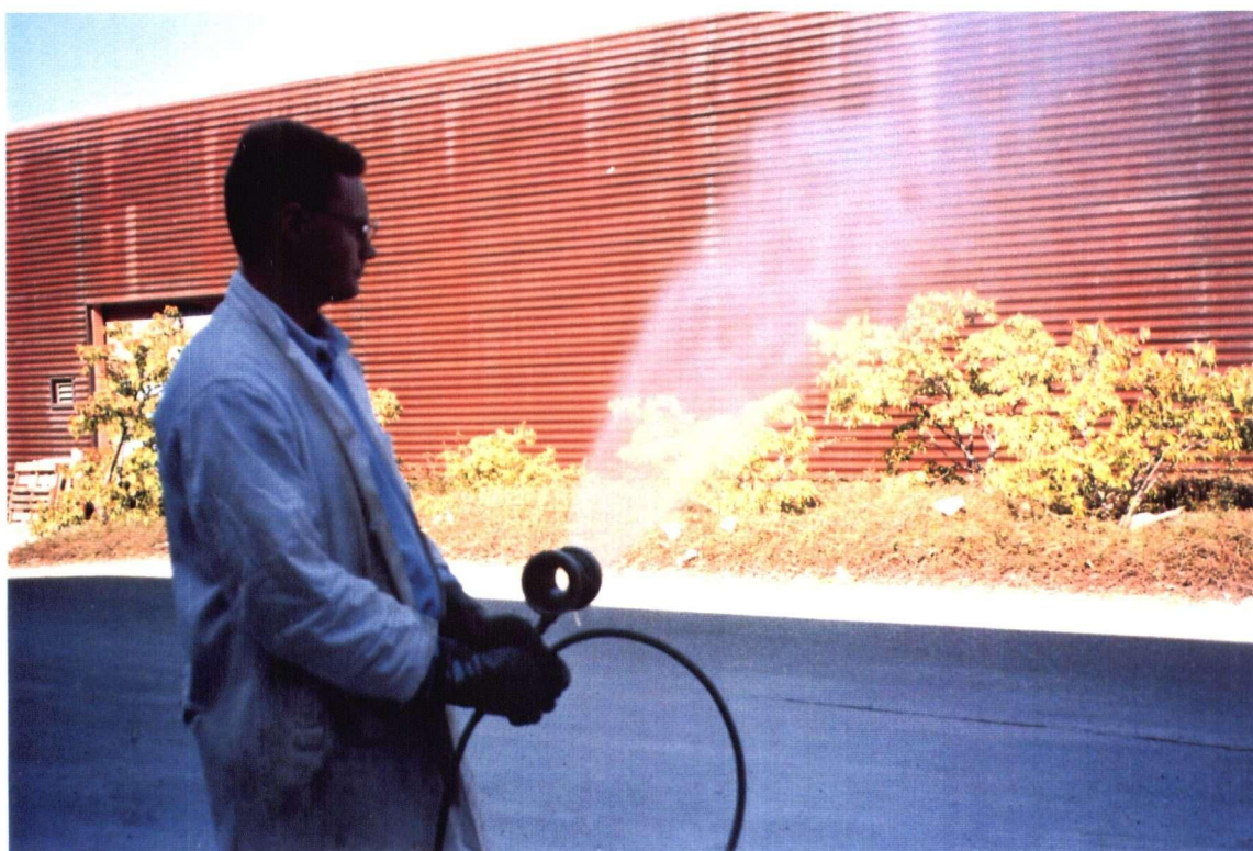
Figure B4 - Because water is injected at a high pressure through a small orifice, a water mist is created.
