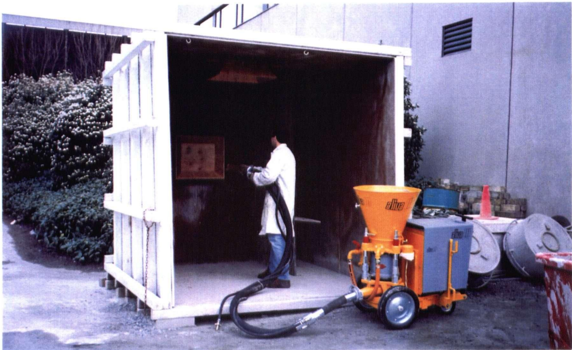
Figure 3.1 - Schematic view of the rebound chamber and the position in which the shotcrete panels were produced.
