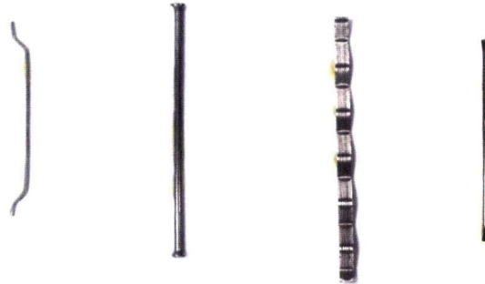
Figure 2.1 - Different steel fiber geometries presently available in the market for concrete and shotcrete reinforcement.
