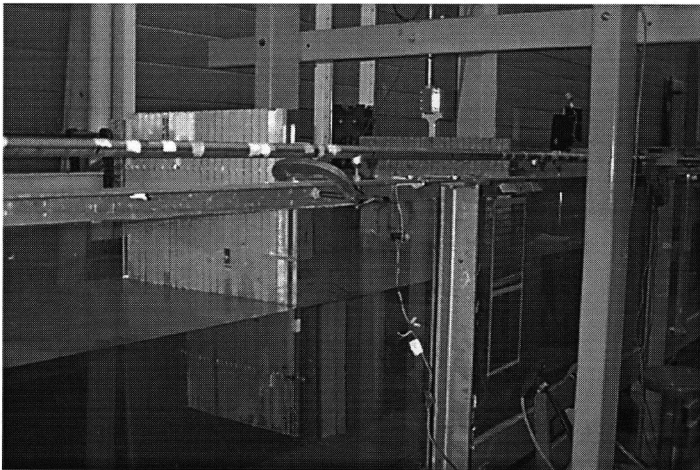
Figure 6. Views of the double barrier in the flume.
