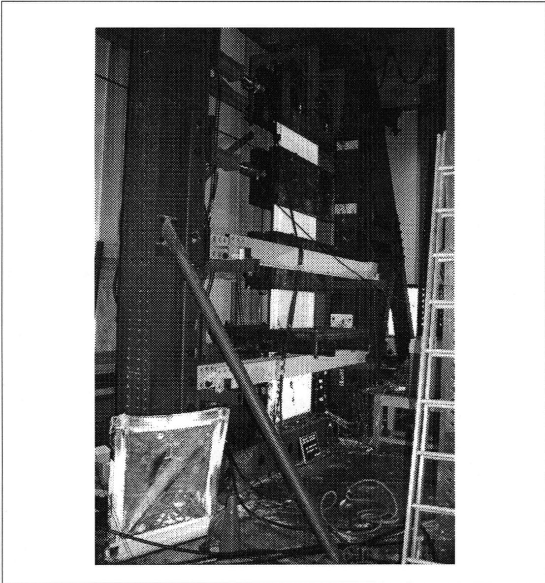
**FIGURE 5.1:** Photograph of specimen SPSW4 within the test frame
