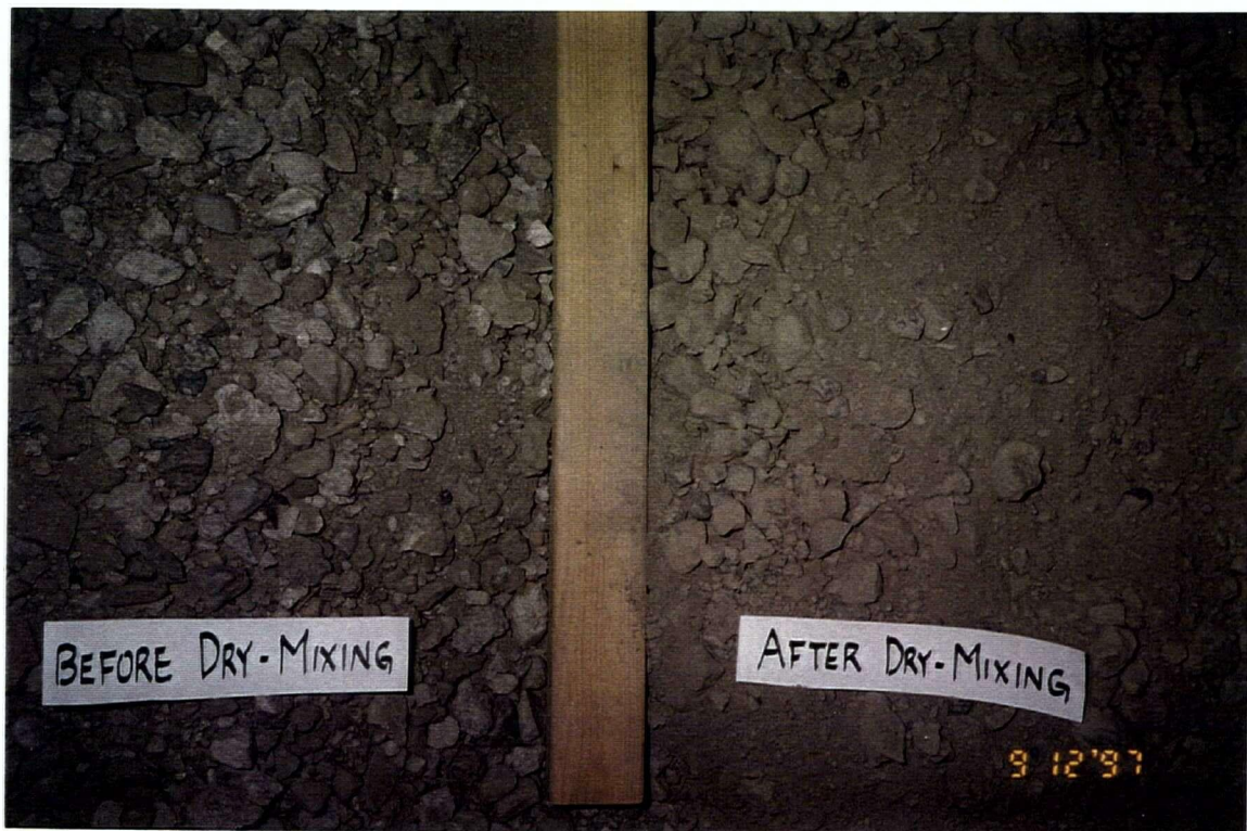
Figure 4.6 Comparison of aggregates before and after 25 min of dry-mixing.
