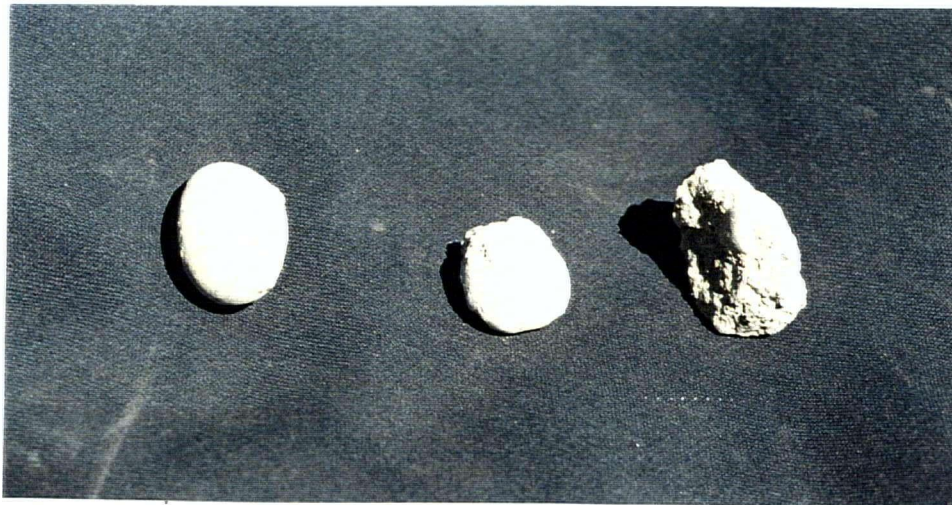
Figure 4.3 Particles with and without attached mortar as taken from recycled aggregates.
