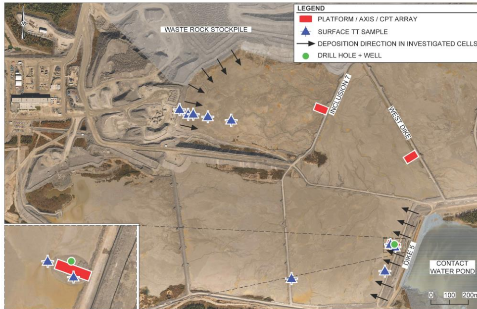
Figure 2. Plan view of the TSF as of September 2013 – CPTs, drill holes and surface sampling locations
