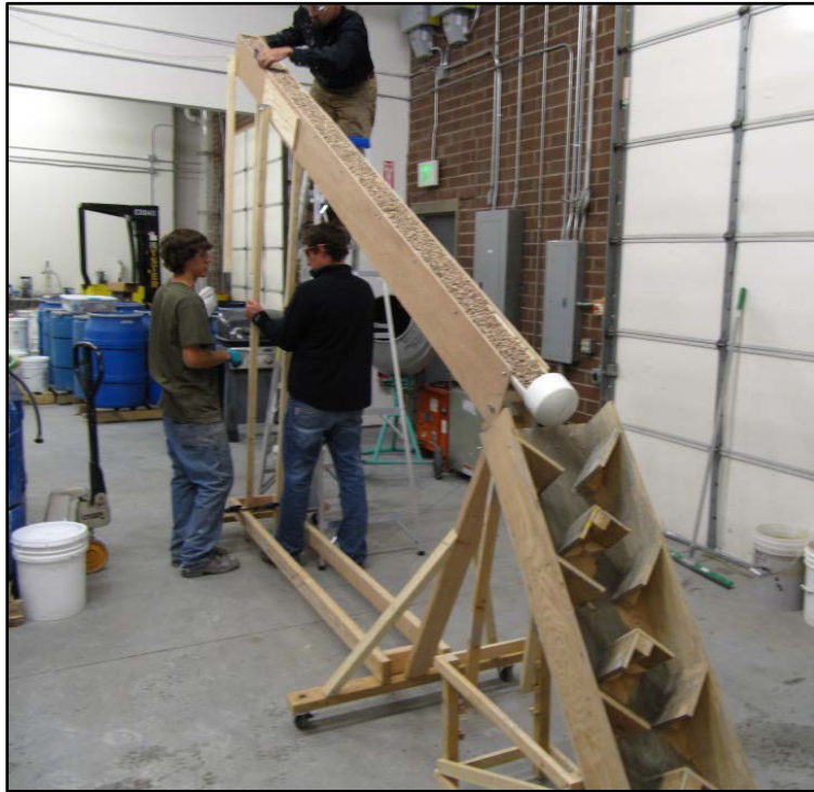
Figure 8. Static Mixing Device with Continuous Feed
