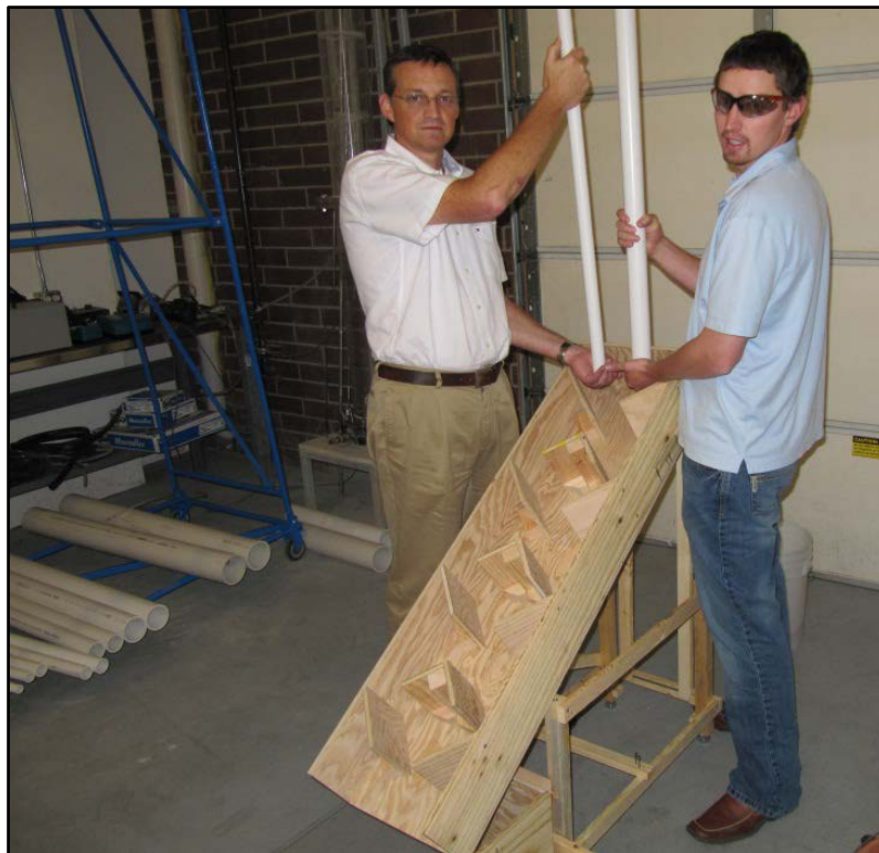
Figure 5. Photograph of Laboratory-Scale Static Mixing Device
