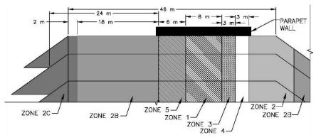
Figure 6:Ultimate TSF Dam Crest Detail
