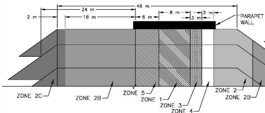
**Figure 6: Ultimate TSF Dam Crest Detail**
